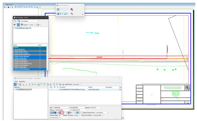
The Detail Callout and construction class elements may be toggled off in the View Attributes. Level Display may also be used to adjust the view.
