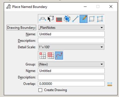
The top row of icons sets the type of boundary. The most commonly used type of **non-civil** drawing boundary for both MicroStation and ORD is "From Drawing Boundary". Non-civil drawing boundaries do not have a scale in the name.
