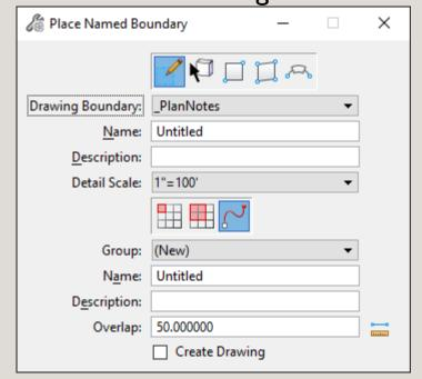
Place Named Boundary By Drawing Boundary > Identify Path Element at Start point
