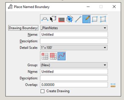
Both MicroStation and ORD can place a **non-civil** drawing boundary "Along a Path". "Path" is a generic term and could mean a complex chain drawn using MicroStation or a civil geometry (alignment) that is displayed as a reference. The MicroStation dialog on the left looks almost the same as the OpenRoads Designer dialog on the right.
