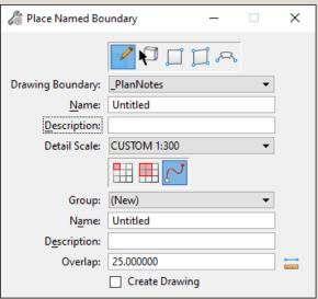
Drawing boundaries are sized according to the Detail Scale selected on the dialog. Use Custom... for any scale not listed. Multiply the scale value in inches by 12 to get the scale factor. For example, 1''=25' is the same as  $1:300 (12\times25=300)$ . Select 1''=100' first, before setting a Custom scale.
