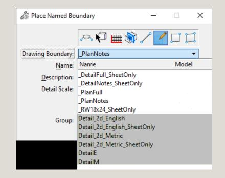
When the type of boundary is set to "From Drawing Boundary", both MicroStation and ORD provide the same list of five (5) ODOT non-civil drawing boundary seeds. ODOT seed names begin with an underscore so that ODOT boundary seeds sort to the top of the list. Don't use boundary seeds that don't have an underscore in the name.
