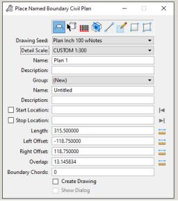
Drawing boundaries are sized according to the Detail Scale selected on the dialog. Use Custom... for any scale not listed. Multiply the scale value in inches by 12 to get the scale factor. For example, 1''=25' is the same as  $1:300 (12\times25=300)$
