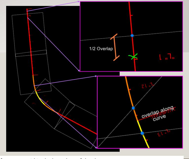
Boundary edges are only perpendicular to path if no curve within the boundary of the sheet.
