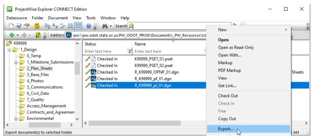
In the picture above, the ProjectWise Explorer is open to the K99999 project in the User Training folders with the folders expanded on the left side. The active folder is 2\_Plan\_Sheets. R\_K99999\_pl\_01.dgn is selected and highlighted blue. Its blue MicroStation icon shows the white tree glyph indicating that it has reference attachments. The right-click menu is open and the "Export" command is highlighted blue.
