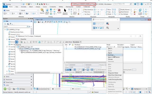
The picture above shows MicroStation open to the plan sheet (.dgn). The References dialog is open at the right showing the reference hierarchy. The Default model is selected in the Hierarchy list and highlighted gray. You can see the permanent address in the "dms" folders in the reference details on the right side. A right-click menu is displayed and Exchange is highlighted blue. The next picture below shows the result of making an exchange.
