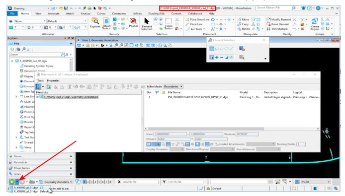
The picture above shows MicroStation open to the Geometry Annotation model of the "CAD base" file in the "export" folder. A red rectangle in the title bar surrounds the path and name of the open (.dgn) file in the "export" folder. A red arrow points to the Previous Model pick list. Using the Previous Model button is the quickest way to transfer back into the plan sheet file.
