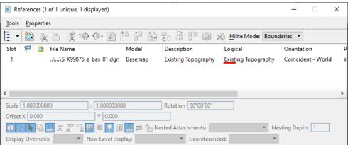
When the plan sheet is printed using the Design\_11x17 or Sheet\_11x17 print style, the plans.tbl pen table is automatically attached. Existing elements are screened to 50% black and appear gray-colored, while the design elements appear dark black.
