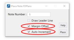
The Roadway bubble tool places numbered circular bubbles. When "Auto Increment" is checked the number will increase by one after a bubble is placed and is used to quickly place a series of sequentially numbered note bubbles.
