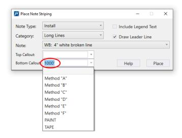
The Place Note Striping tool includes optional top and bottom callouts that can be placed with the bubbles. Predefined callouts can be selected from the callout drop down menus or custom values may be entered as illustrated in these images.
