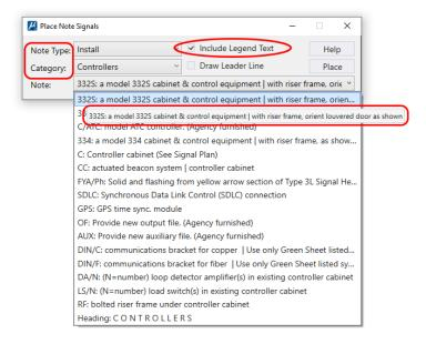
When the "Include Legend Text" checkbox is enabled, the legend text is placed to the right of the bubble as shown below.
