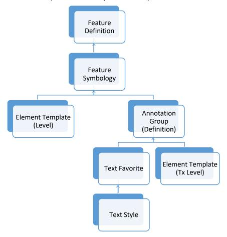
Each category of feature definition has a feature symbology or element template assigned in the properties to control the display of the element. Though "Alignment" and "Linear" feature definitions allow the assignment of different *linear* symbology and *profile* symbology, ODOT uses the same feature symbology for linear and profile display for both categories.
