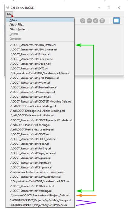
It is not necessary to open the cell library to use standard cells. Typical usage, is to place standards cells using an ODOT discipline ribbon workflow. When items are selected from an ODOT ribbon workflow, the cell is found within the appropriate cell library and used by the software.
