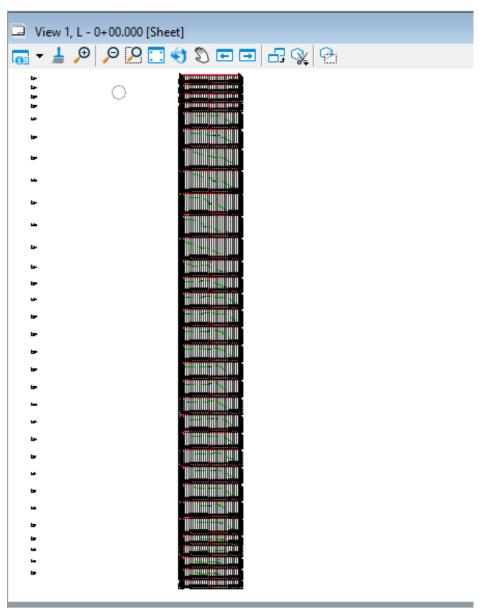
Drawing models are created for each section, then the drawing models are all attached in a stack to the one sheet model.
