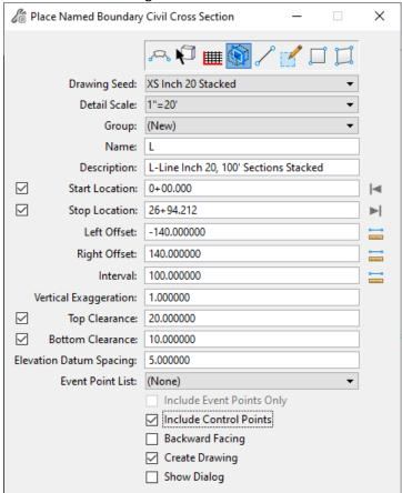
Left-click 3 times – then – wait while the drawing- and sheet-type models are created! Longer if the interval is set to 50 or 25.
