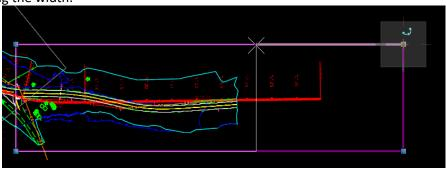
Return to the sheet model to see the results. The reference to the sheet can be moved for a different alignment in the sheet.
