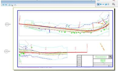
To adjust the named boundaries, use the section callout icon at the left to select "Open Design Model" – this will open the Default model, with the view rotated to align with the sheet.
