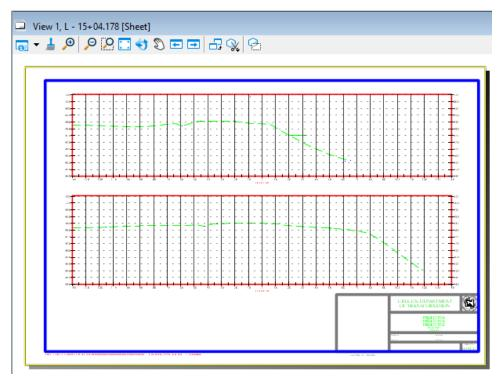
Sheet models are named for the lowest station value displayed in the sheet. Sections are displayed in a stack on each sheet, beginning above the title block. The title block contains a Sheet Number cell that displays the Sheet Number from the sheet model properties.
