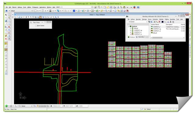
If you do a little **HORIZONTAL ALIGNMENT TRACKING**, or zoom into the plan graphics, you'll find that the area where the ROW was imported is around **Station 490+00** along the mainline alignment.
