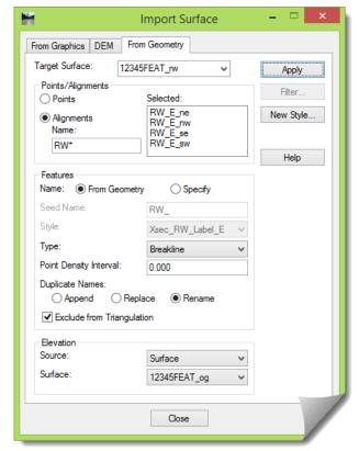
The only unique item of note about this tool is the way it establishes the **Elevation** when the **Source** is set to **Surface** as mentioned earlier. So after this command is used, the next step of finalizing the elevations along the new Right-of-Way features has to be done using the **DRAPE SURFACE** tool under **SURFACE** > **DESIGN SURFACE**.
