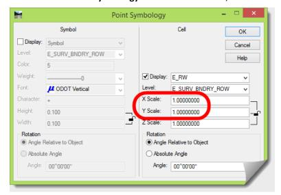
Notice the **X Scale:** and **Y Scale:** settings. They are both set to **1.00**. This is fine for a cross section display at 1H:1V. But if a **Vertical Exaggeration** is applied to the cross sections then the Cell, in order to be proportional, has to be scaled to compensate for the **Vertical Exaggeration**. It's time for some practice.
