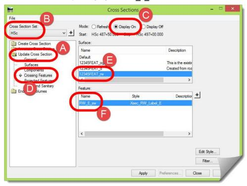
5) [Apply] this command and see if the ROW marker appears on the cross section You should be seeing something like this on the cross section.
