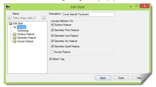
Selecting the **Surface Feature** leaf (which defaults to opening the **Settings** leaf) exposes the specific Surface **Display** settings.
