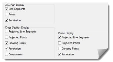
The main thing to understand here is that InRoads has the capability to place information contained in the surface DTM into the Plan, Profile and Cross Section displays. If you have that desire, or expectation, the **Style** has to support that desire. If the **Style** is not optioned or configured to present itself in that environment it either has to be edited or acknowledged that it is not designed to do that.
