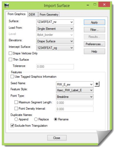
6) [Apply] the command and the dialog box will collapse. Follow the Prompts to > Identify element and then > Accept/Reject the selection.
