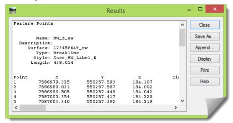
These elevations can be checked to be in the ballpark either by your understanding of the terrain elevations or by doing some quick **Tracking** along the surface in that area.
