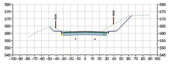
There are two parts to this 'intelligent' equation – the 3D **Feature** stored in the surface, and the InRoads unique **Style** that provides that **Feature** the intelligence to understand what it needs to do in Plan, Profile or Cross Section.
