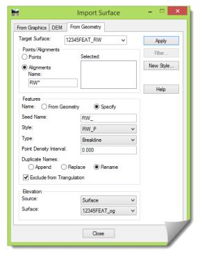
• PLACE FEATURE — This is another tool, found as part of the SURFACE > DESIGN SURFACE tool set, which provides the capability to enter surface information directly into a DTM.
