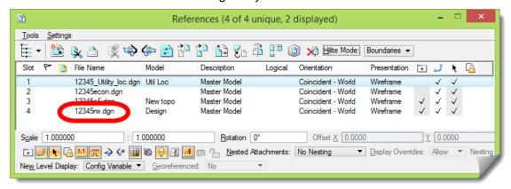
The references contain information about the base drawing, utilities, existing contours and the right-of-way. The one key reference used during this module is the **12345rw.dgn** that contains the Right-of-Way graphics. We will use these graphics as a launching point toward placing ROW markers on the Cross Sections for this roadway.
