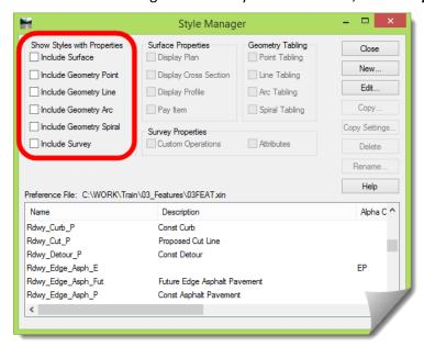
Opening a specific **Style** continues to reveal its association with the 3 main file types – **Surface**, **Geometry** and **Survey**. For this module the focus will be on the Surface configuration since that is the route that will be taken to get the Right-of-Ways displayed on the Cross Sections.
