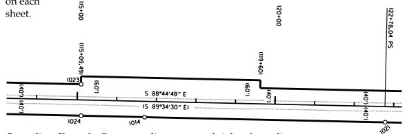
25. Centerline: Show the Recovery alignments and right-of-way lines. (Multiple alignments should be noted in different line styles and/or have unique labeling). Show the alignments with stationing, all centerline control points and PIs. List the coordinates at PIs, POTs, angle points and the ends of the alignment only.
