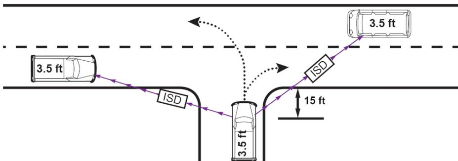
Intersection sight distance (ISD) measures a line of sight from the height of driver's eye (3.5 feet), seated 15 feet back from the fog line or edge of the traveled way, to the right and to the left, to an object in the highway that is 3.5 feet high.
