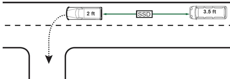
Stopping sight distance (SSD) is measured from the height of a driver's eye (3.5 feet) to an object 2 feet high or more in the roadway.
