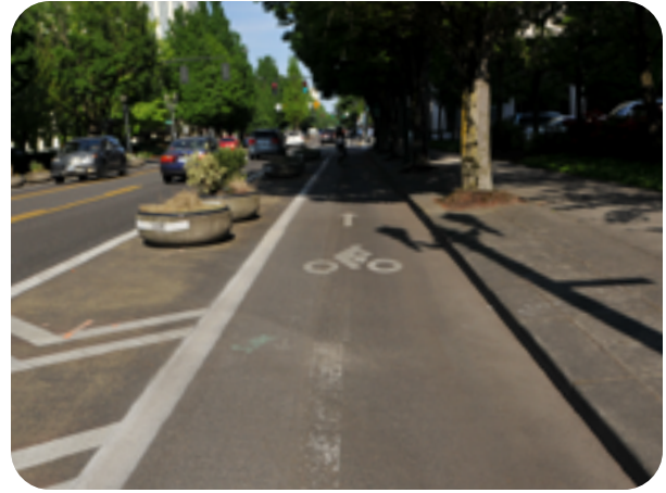
Planters and pavement markings create a larger buffer for the bike lane on Lloyd Blvd. in Portland. Photo from Metro.
