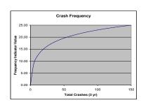
The crash rate indicator,  $IV_{Rate}$ , is a value between 0 and 25, also determined by using a logarithmic distribution based on the following crash rate calculations. Again, the <u>maximum</u> indicator value of 25% is obtained when the crash rate reaches seven crashes per million entering vehicles.
