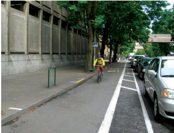
Figure 900-9: Parallel parking lane as street buffer
