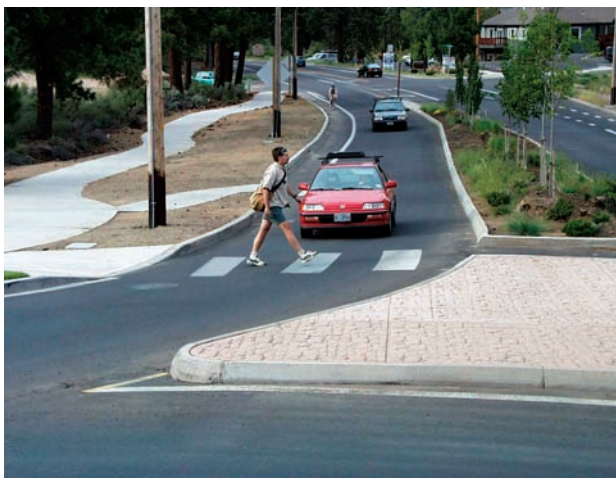
Pedestrian crossing to splitter island at roundabout
