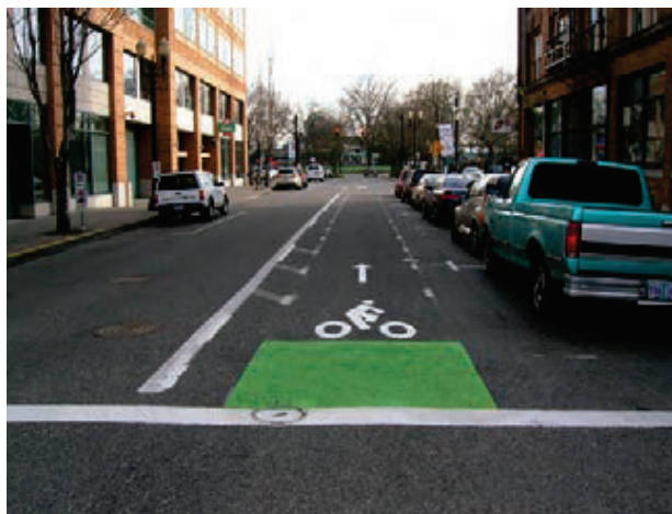
Buffered bike lane markings can act as a street buffer or as a buffer from parked cars in the sidewalk buffer zone.
