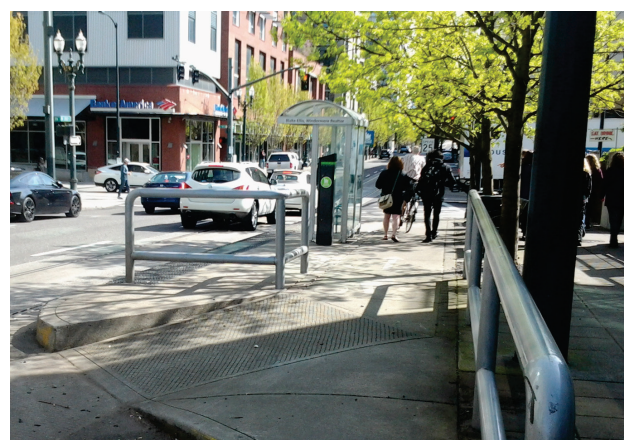
Integrated boarding platform may result in pedestrians blocking bike lane
