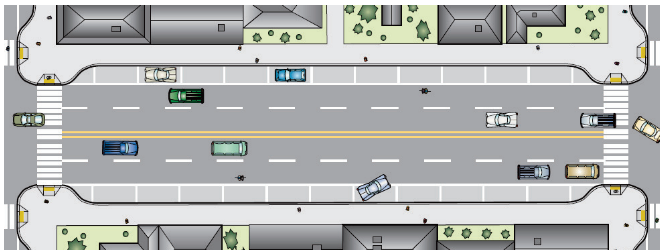
Figure 5-43: Roadway designed with curb extensions and integrated parking lanes
