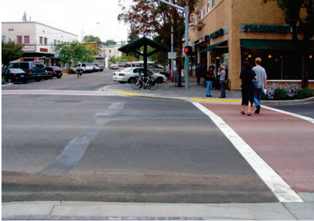
Curb extension provides room for bike parking
