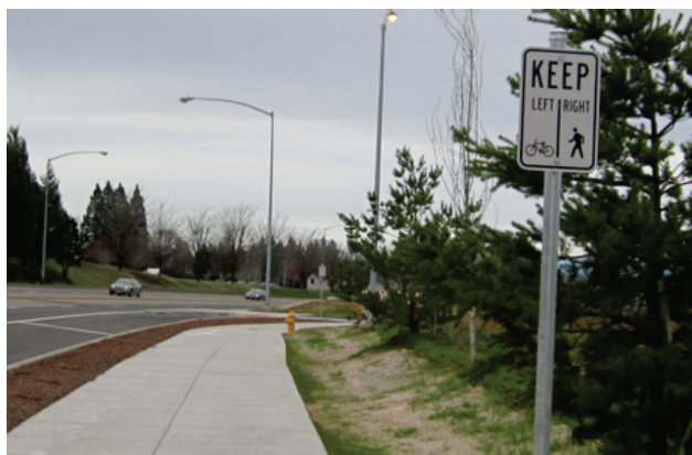
Shared use path with sign indicating which side of path each mode is expected to use. However, users are allowed to mix.
