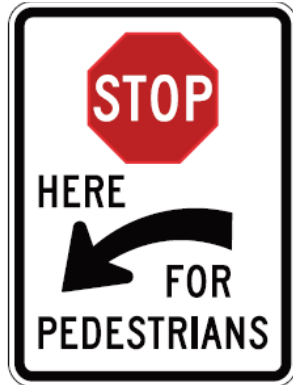
Figure 5-32: Sign R1-5c are placed adjacent to the stop bar
