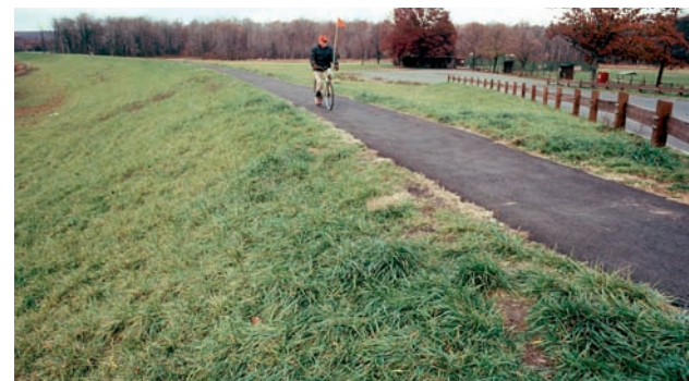
Gentle grassy slope eliminates the need for railing
