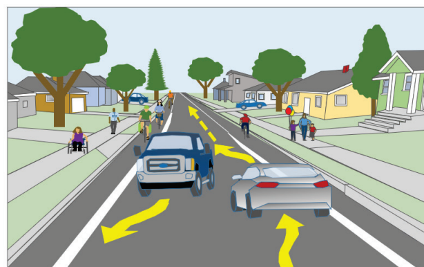
Edge Lane Yield Street (sufficient space for vehicles to pass without encroaching into bike lanes)
