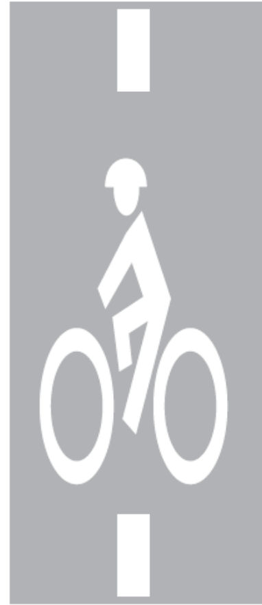
Figure 1-52: Bike symbol for loop detection placement
