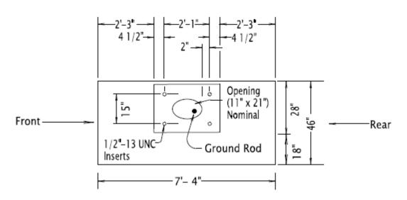
Note: Additional details for installing the controller cabinet on this foundation are shown in standard drawing TM454.
