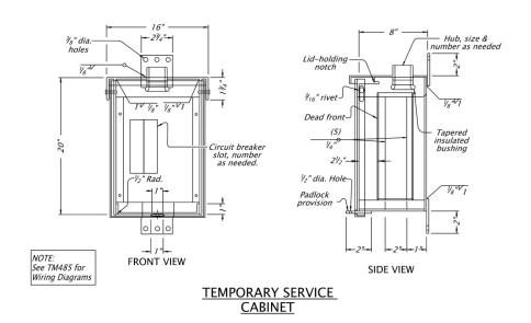
Includes circuit breakers, contactors, test switches, neutral and ground bars as shown in standard drawing TM485
