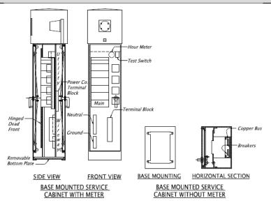
Includes circuit breakers, contactors, test switches, neutral and ground bars as shown in standard drawing TM485
