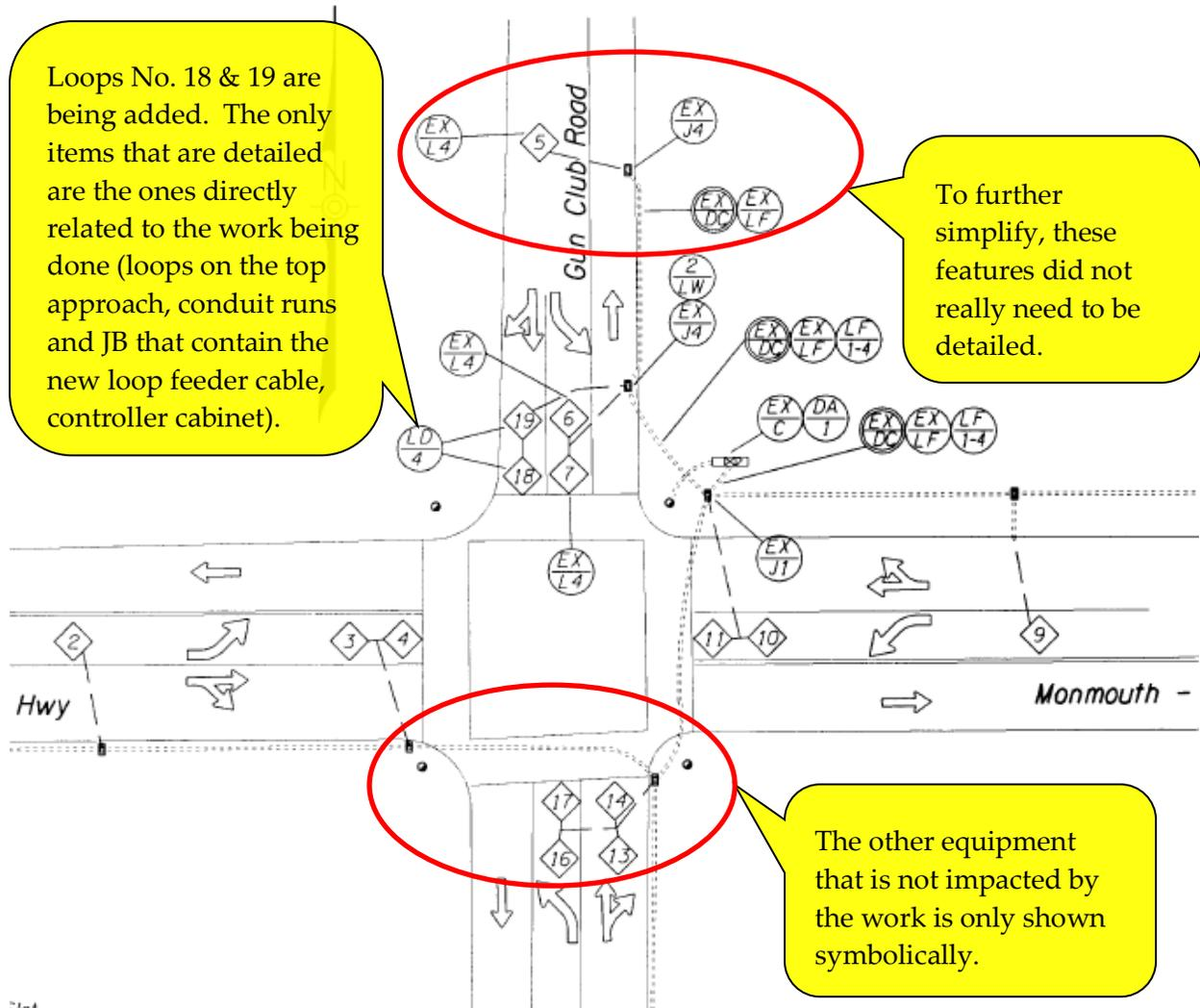
Figure 22-4 | Detailing Equipment Not Impacted by the Work (Avoid this Method)
