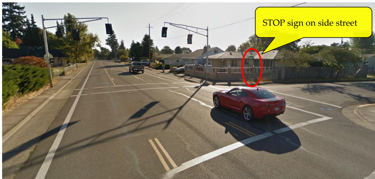
Figure 14-5 | Pedestrian Signal Installed at Intersection (Half-Signal), Prohibited
