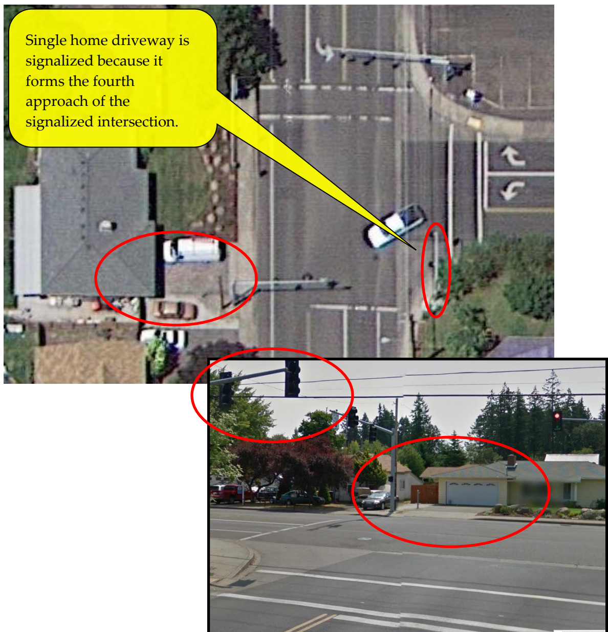
Figure 5-15 | Signalized Driveway Example
