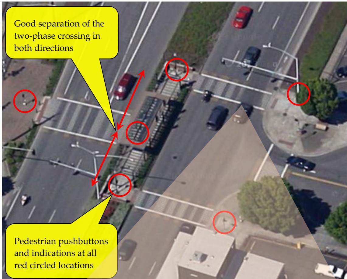
Figure 5-9 | Two-Phase Pedestrian Crossing (Staggered Crosswalk Alignment) Example 1
