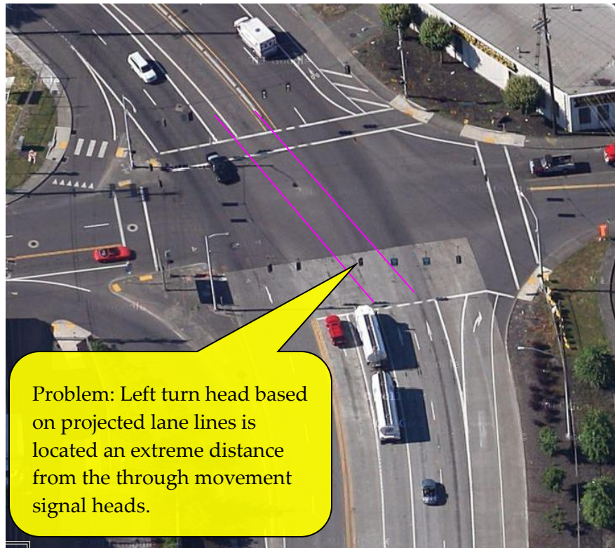
Figure 5-31 | Horizontal Curves and Signal Head Alignment, Example 2
