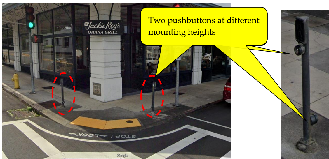
Figure 5-94 | Deviation to Vertical Reach Example
