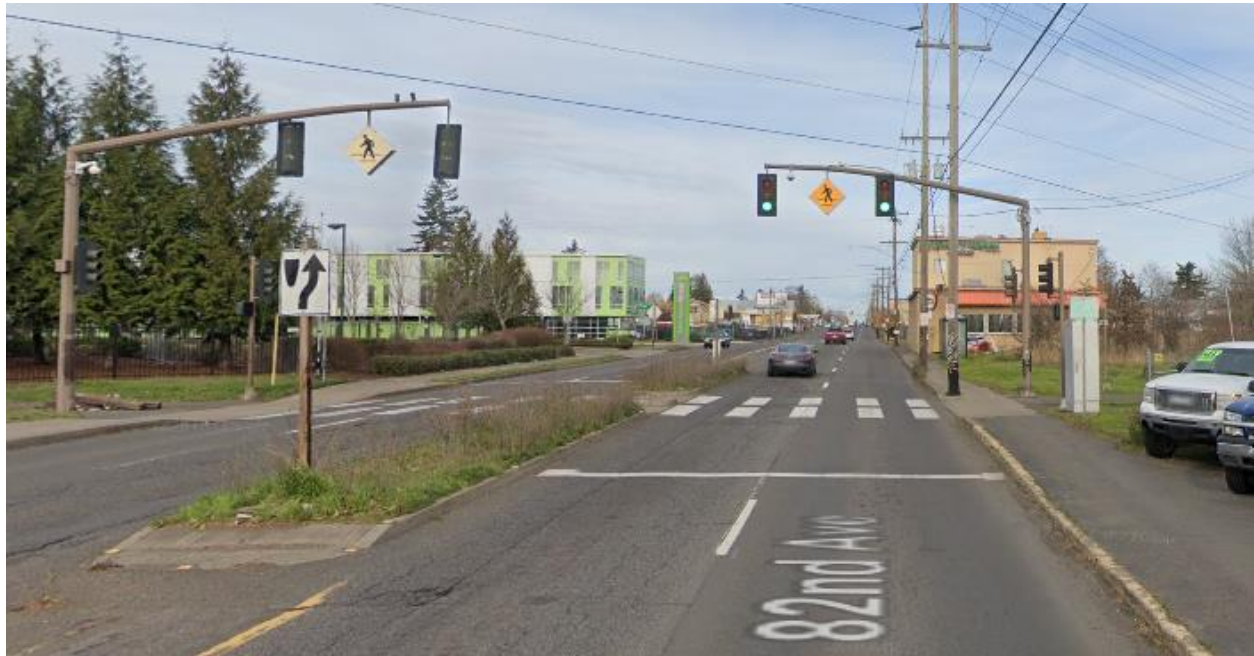
Figure 14-3 | Pedestrian Signal Installed Mid-Block, Example 3
