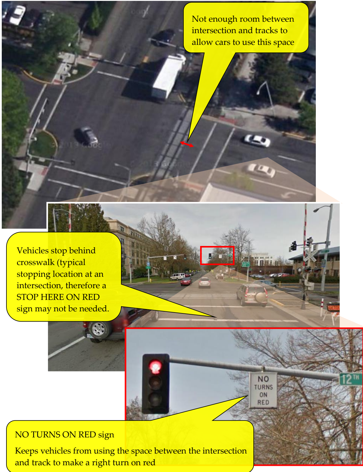
Figure 16-4 | VCOI is Not Required, Example 1
