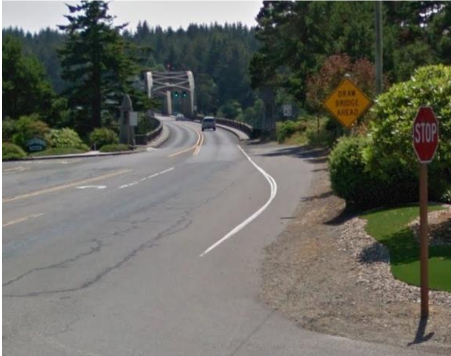
Figure 24-7 | Non-Compliant Existing TCD: Outdated Signs, Example 2
