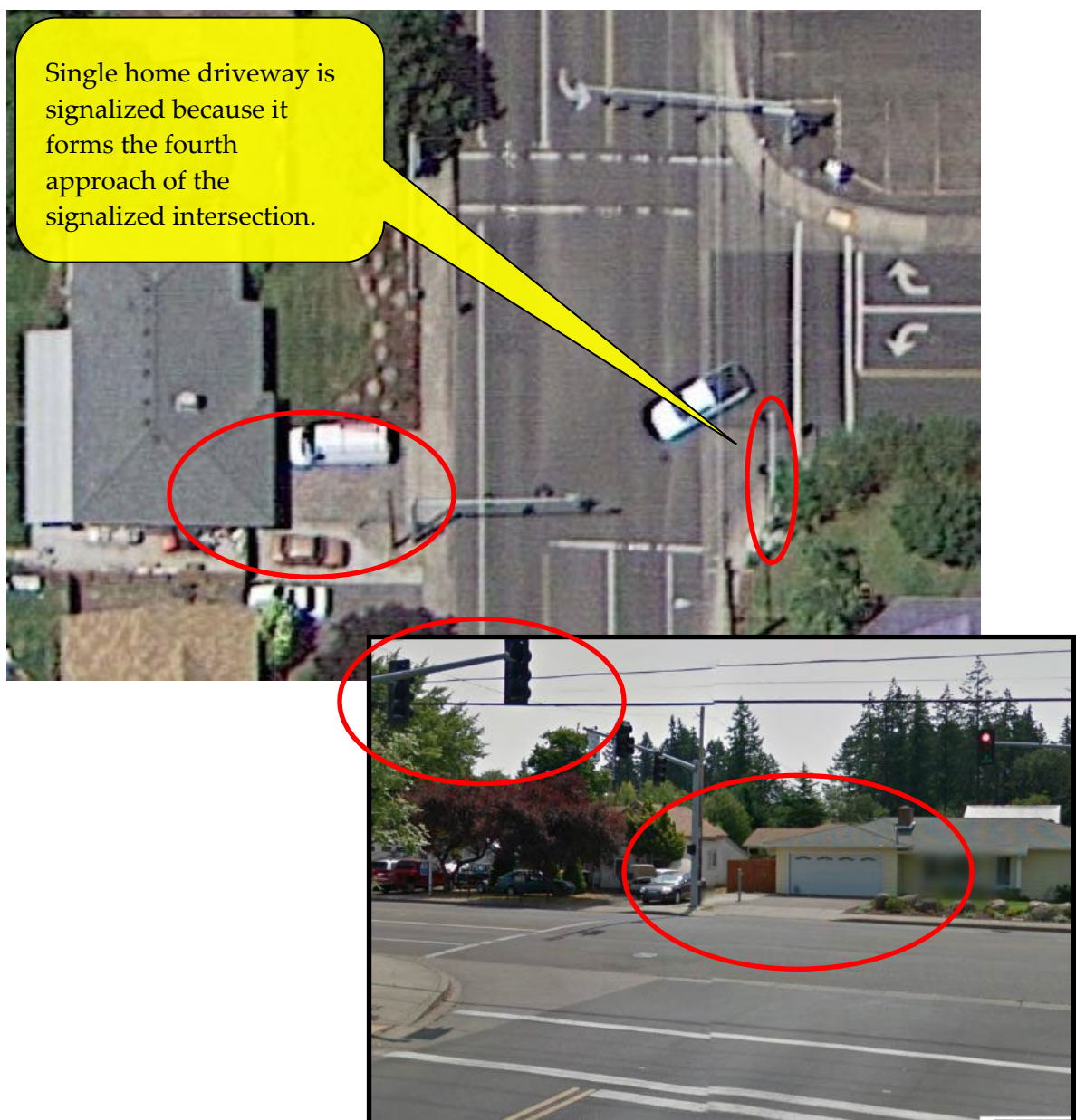
Figure 5-15 | Signalized Driveway Example
