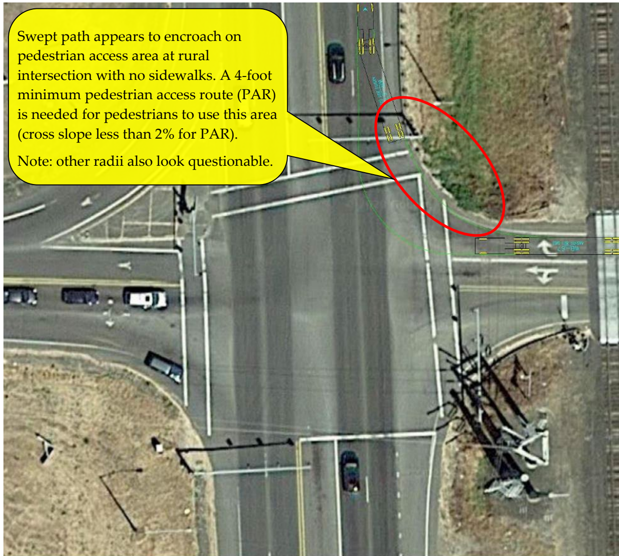
Figure 5-21 | Truck Turning Templates – Verifying Right Turns
