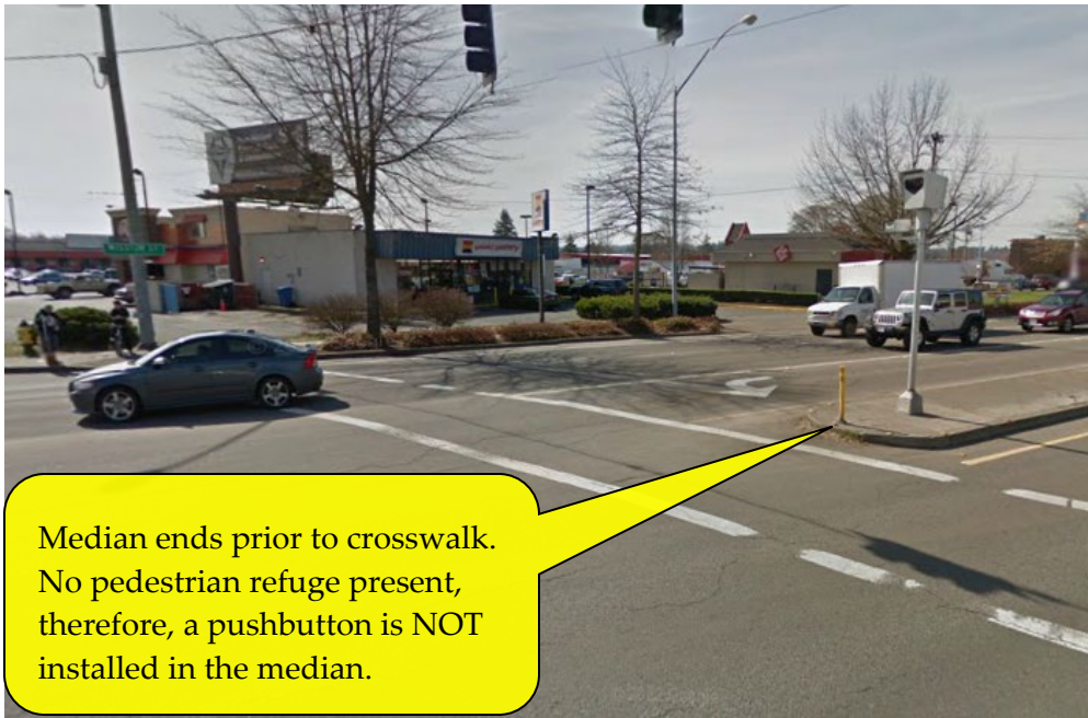
Figure 5-12 | Single Phase, One Stage Pedestrian Crossing (Recommended Crosswalk & Median Design) Example 2
