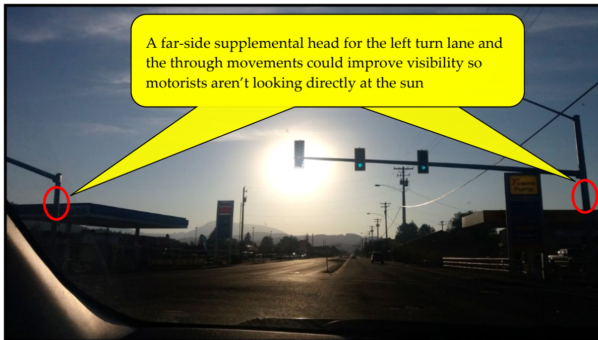
Figure 5-51 | Supplemental Signal Head Placement – Sun Glare Example
