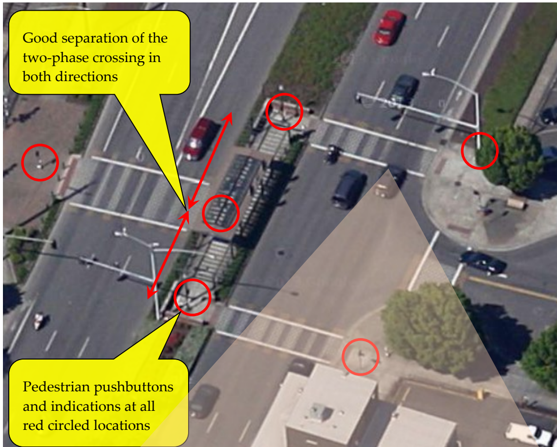
Figure 5-9 | Two-Phase Pedestrian Crossing (Staggered Crosswalk Alignment) Example 1
