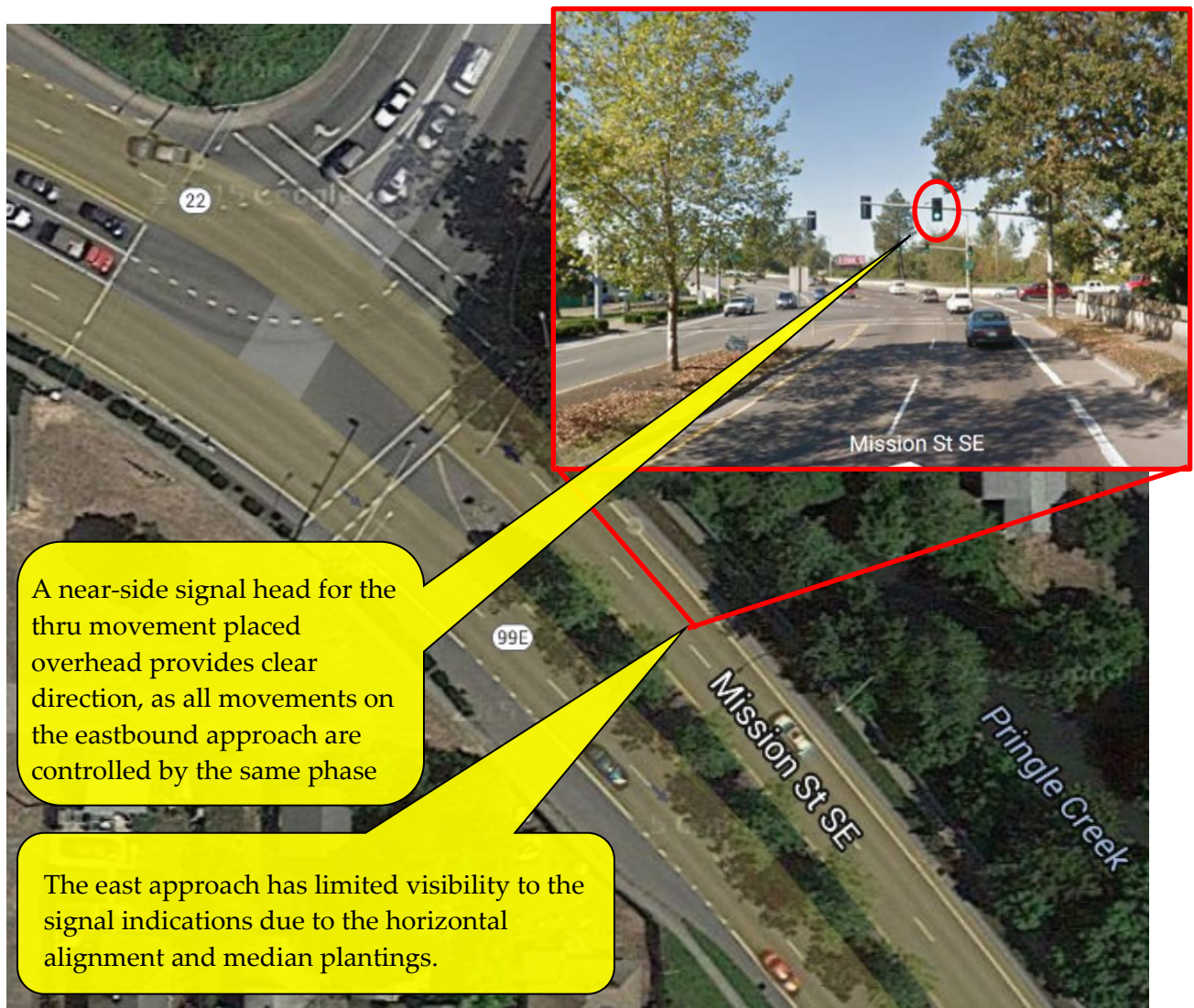
Figure 5-47 | Supplemental Near-Side Signal Head Placement: Example 1, Recommended
