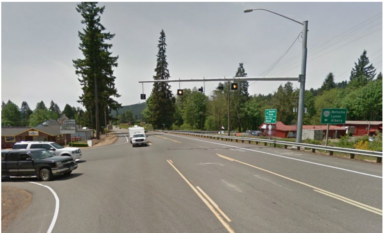
Figure 12-33 | Intersection Control Beacon, Mast Arm, Example 2
