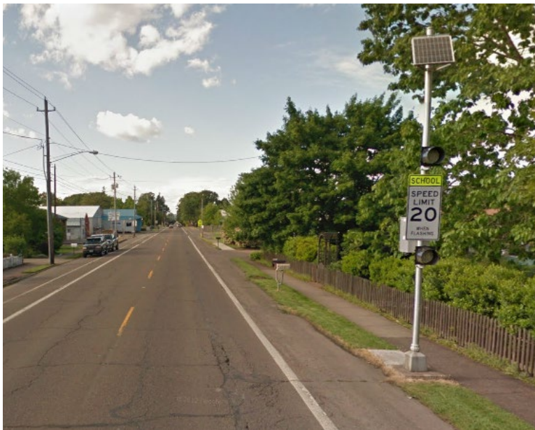
Figure 12-29 | Speed Limit Beacon for School Speed Zone
