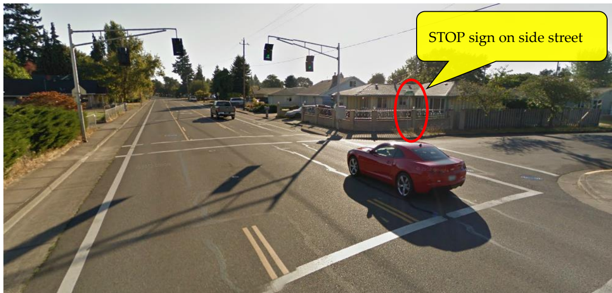
Figure 14-5 | Pedestrian Signal Installed at Intersection (Half-Signal), Prohibited
