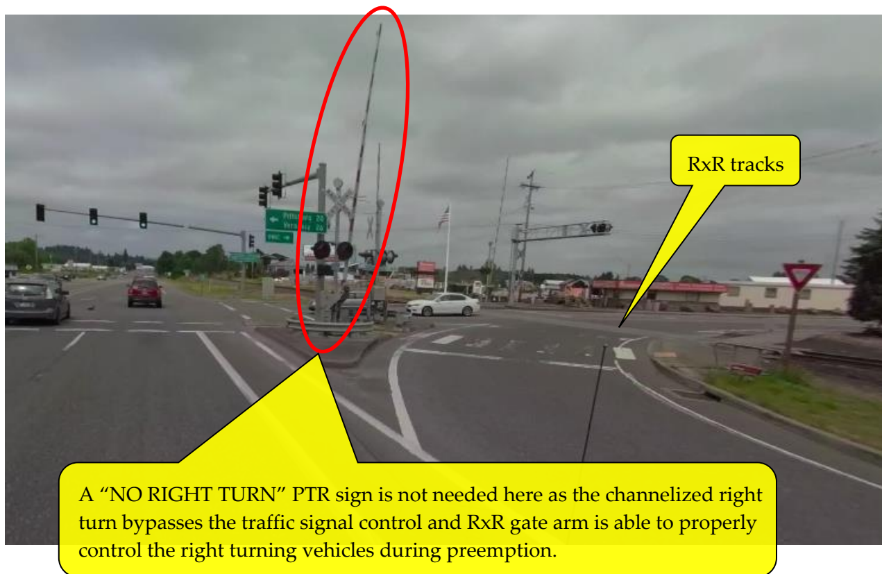
Figure 16-24 | Omitting the Part-Time Restriction Sign Example 4
