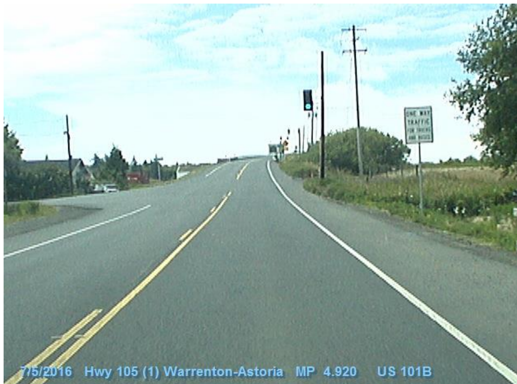
Figure 24-5 | Non-Compliant Existing TCD: Single Advance Signal Head, Example 2
