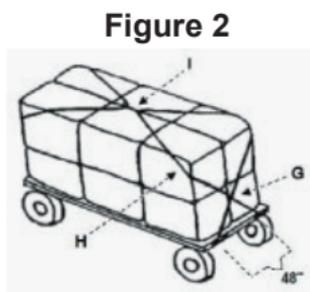
**Lateral Tiedowns** — Each tiedown must have a minimum working load limit of 4,000 lbs. Multiple tiedowns may be substituted if each has a load limit of 625 lbs., with a combined working load limit of 4,000 lbs. or more. Tiedowns less than 2 inches in width or diameter must include V-boards. Vehicles 32 feet or less long require one tiedown in the center of the length of the vehicle. Longer vehicles need two tiedowns – at one-third and two-thirds the length of the vehicle.
