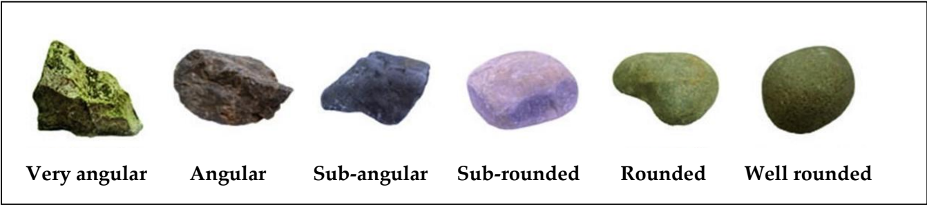
Figure 5-5 Particle Shape for Coarse-Grained Soil Particles
