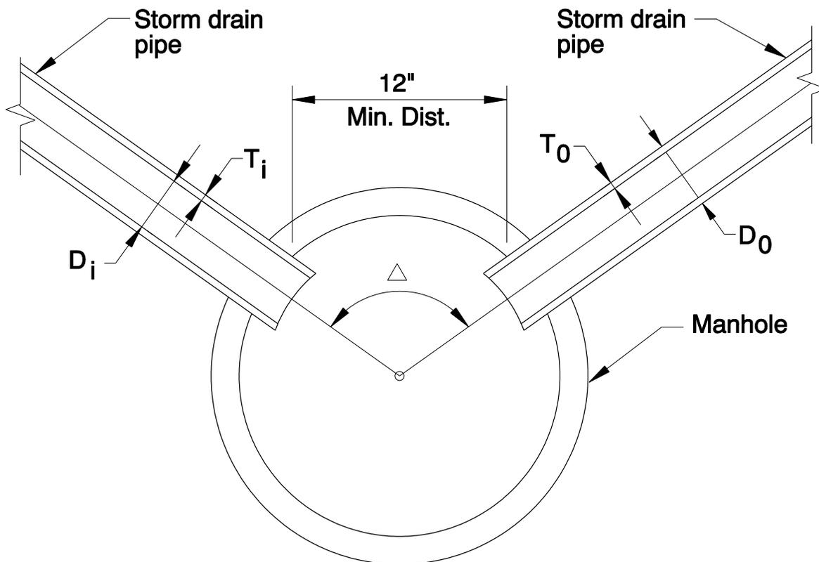
**Figure 1 Manhole Sizing**
