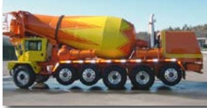
They are commonly used in the construction, waste management, and commodities hauling industries. SHVs use closely-spaced axles that raise or lower as needed for weight, and can result in heavier loads concentrated over a shorter length.
