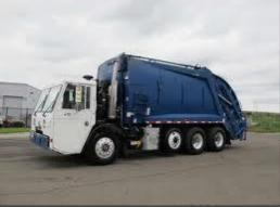
The second SHV model is the SU5, which a five axle vehicle with a gross vehicle weight of 62,000 LBS (31 tons).
