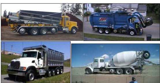
The third SHV model is the SU6, which is a six axle vehicle with a gross vehicle weight of 69,500 LBS (34.75 tons).
