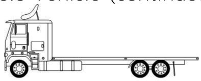
Front Overhang – In excess of 4 feet for non-divisible load, subject to maximum overall length and legal rear overhang.
