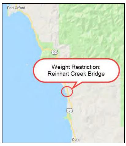
Stop traffic and straddle centerline when crossing this bridge, when exceeding the weight limits allowed. Certified flaggers and signing required.
