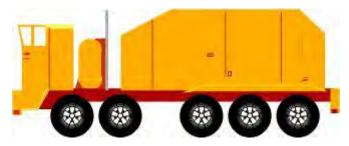
Front Overhang – In excess of 4 feet for non-divisible load, subject to maximum overall length and legal rear overhang.
