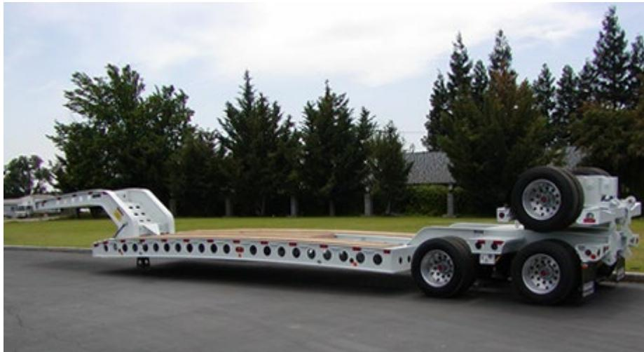
**Pinned Axle(s)** – a separate vehicle pinned to another vehicle adding extra carrying capacity to a vehicle. The additional axle(s) do not pivot from side to side at the connection point or have wheels that steer during turning.
