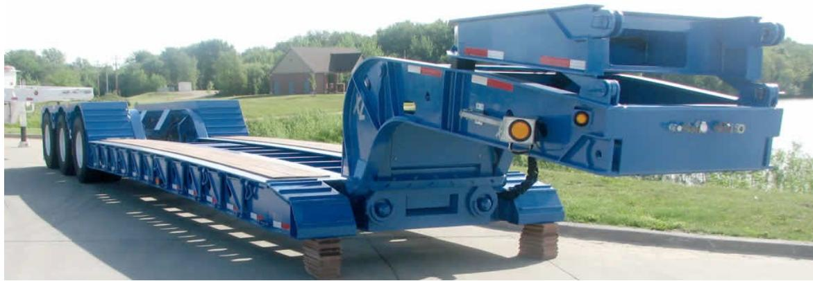
**Flip Axle(s)** – an axle that is bolted or pinned to a vehicle and flips from the closed position on the trailer to a deployed position on the ground extending the length or hauling capacity of the trailer.
