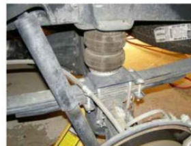
Aftermarket/Secondary Air Suspension (Air Bag Supplements the Primary Leaf Spring Assembly)
