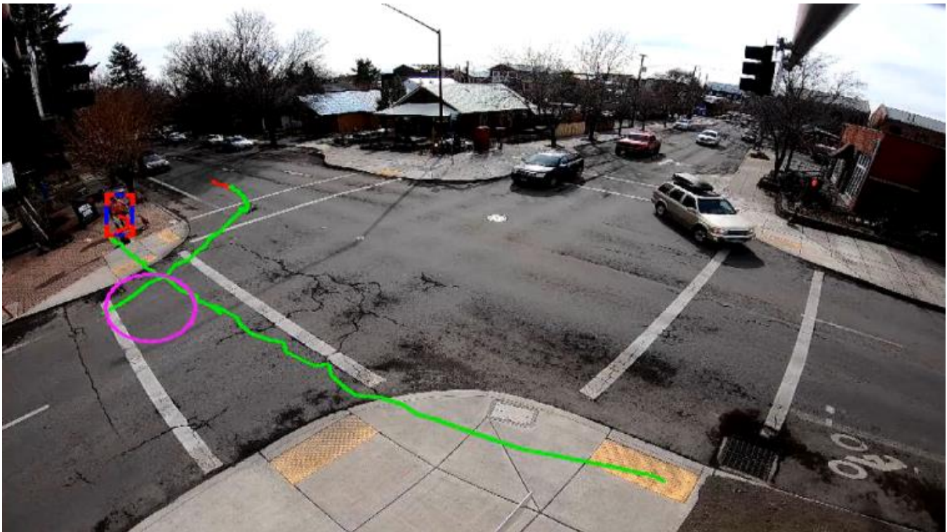
FIGURE 8.6: STREET SIMPLIFIED CAMERA IDENTIFYING A PEDESTRIAN-VEHICLE NEAR MISS EVENT AT NW COLORADO & NW BOND
