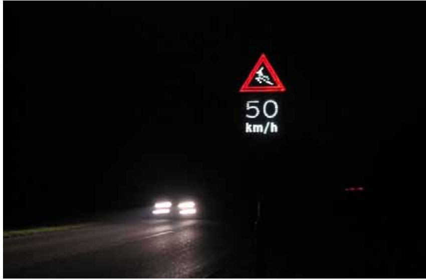
Figure 4.5: Activated warning signal and sign in 't Harde, The Netherlands (Photo: Marcel Huijser/WTI-MSU)
