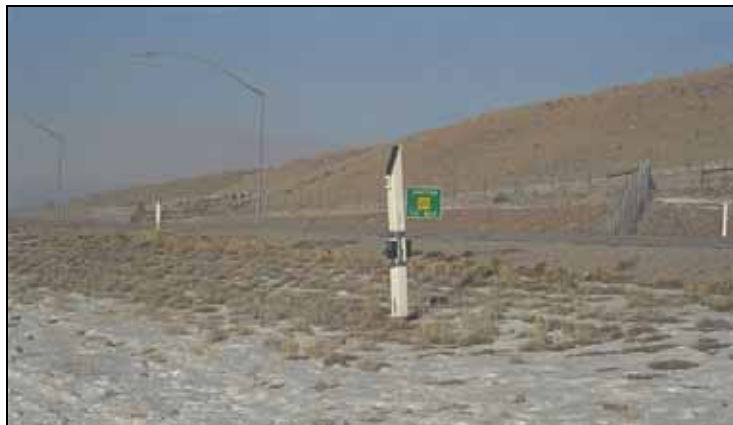
Figure 4.16: Infrared sensors attached to the white posts in the FLASH system at Nugget Canyon, Wyoming, USA (Photo: Bill Gribble/WYDOT)
