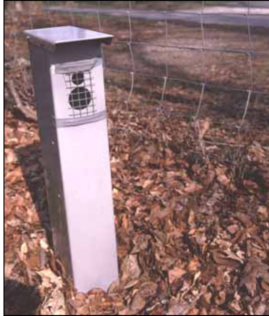
Figure 4.10: Cabinet with infrared sensor in Ugchelen, The Netherlands. The wire in front of the two openings prevents birds from nesting in the box. (Photo: Marcel Huijser/WTI-MSU).
