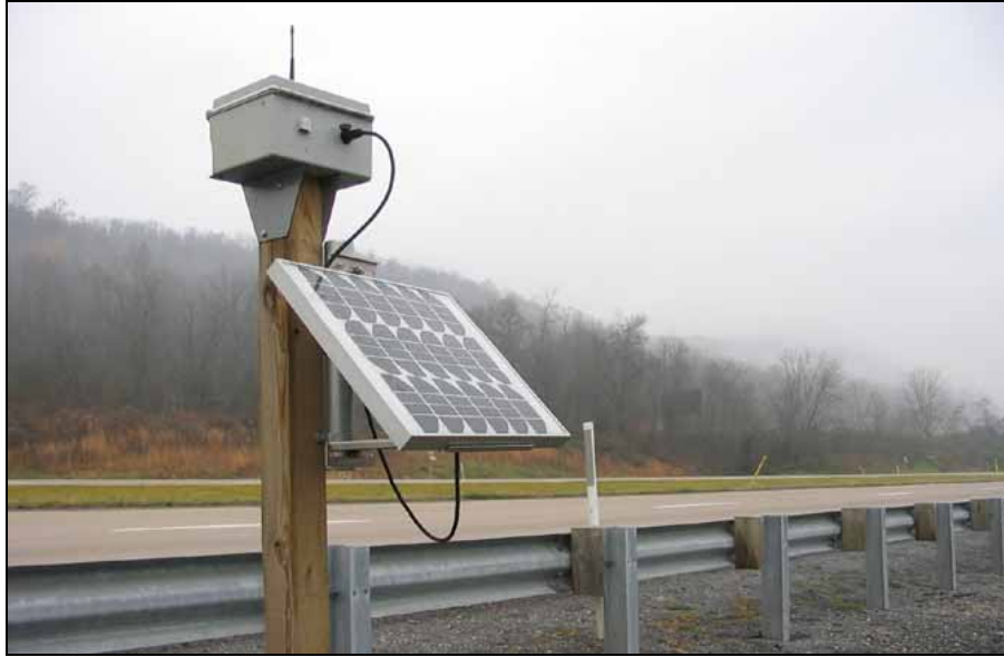
Figure 4.39: Pole with sensors and solar panel in Thompsontown, Pennsylvania, USA (Photo: Marcel Huijser, WTI-MSU)
