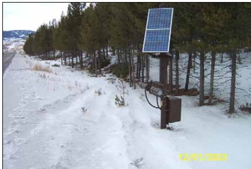
Figure 10.3: Animal detections may reduce or prevent animal-vehicle collisions, but the poles and equipment in the right-of-way form a hazard of their own. Here a car went off the road at the MT site and just missed the pole. However, the damage to one of the sensors was about $2000. (Photo: Jason Norman, MDT)
