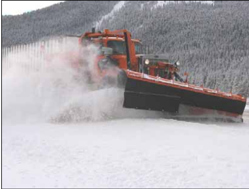
Figure 7.10: Snow spray from a snow plow at the MT site. Depending on the amount of snow spray, how far the snow is thrown into the right-of-way, and the location of the beam, snow spray can trigger the system. (Photo: Marcel Huijser, WTI-MSU)
