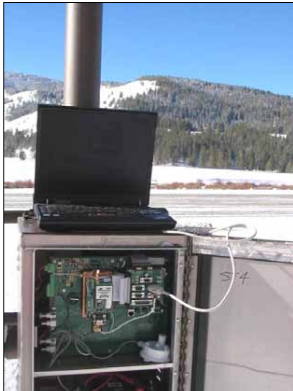
Figure 5.13: Data can be downloaded from the master station at the MT site through a direct connection or a radio link (Photo: Marcel Huijser, WTI-MSU)
