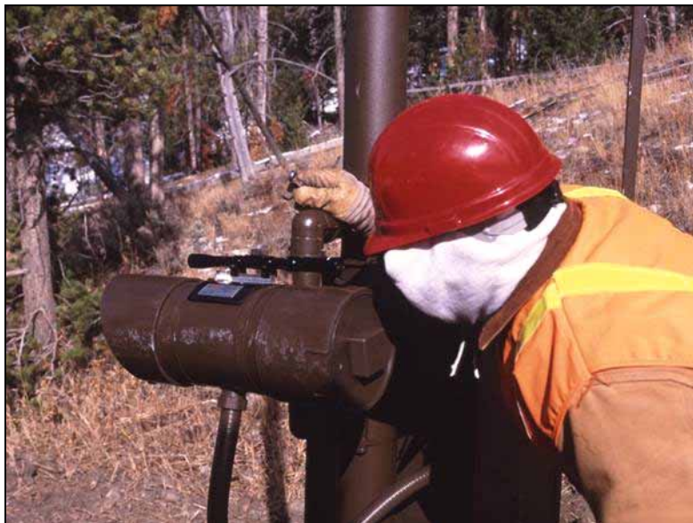
Figure 5.24: Sensors at the MT site were aligned by using a scope (Photo: Marcel Huijser, WTI-MSU)
