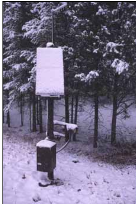
Figure 8.8: Snow may temporarily cover the solar panels. The batteries should have enough power storage to accommodate for such events. (Photo: Marcel Huijser, WTI-MSU)
