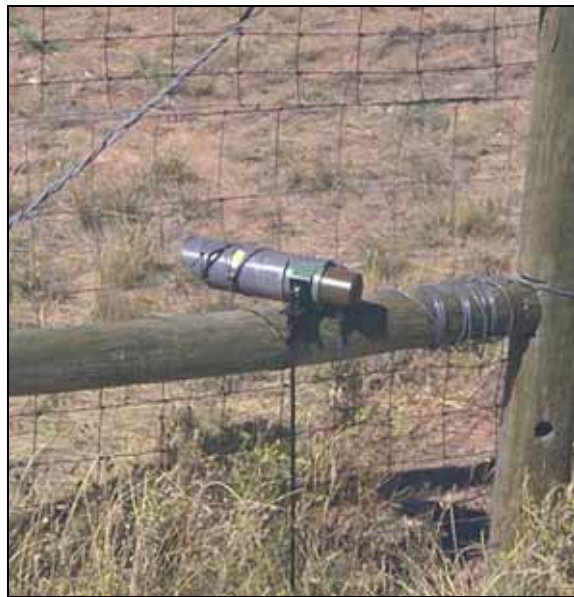
Figure 4.18: Infrared scope for the geophone system at Nugget Canyon, Wyoming, USA (Photo: Bill Gribble/WYDOT)
