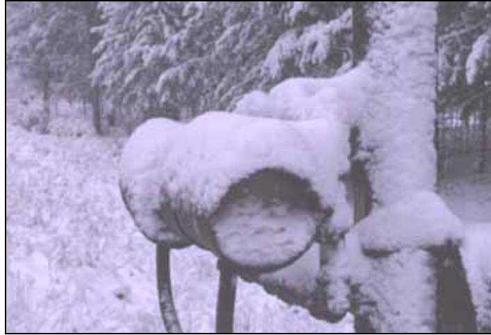
Figure 6.9: Snow and ice build-up on the sensors caused false positives at the MT site (Photo: Marcel Huijser, WTI-MSU)
