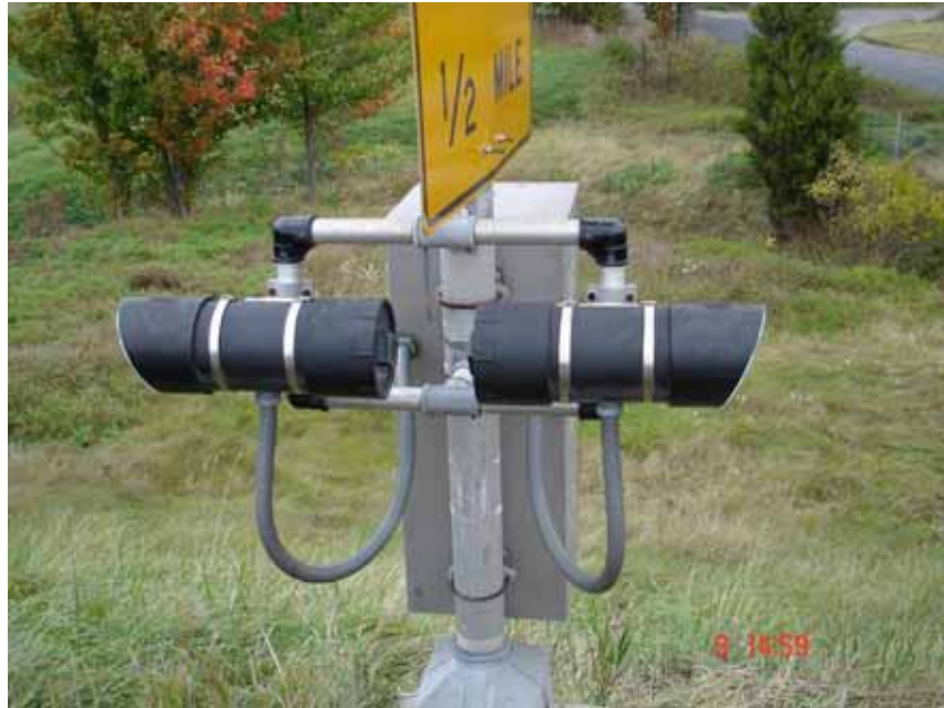
Figure 6.2: Typical receiver/transmitter station showing beam tubes and mounts at an Indiana site (see Chapter 4 for details on the Indiana site) (Photo: Lloyd N. Salsman, STS)
