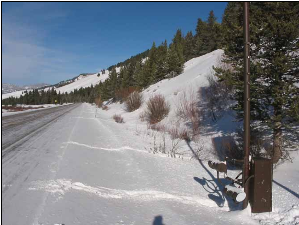
Figure 7.6: Investigation for potential blind spots. The tracks indicate where human models passed through the beam. (Photo: Marcel Huijser, WTI-MSU)
