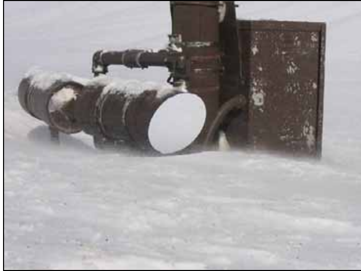
Figure 8.6: Snow accumulation at the MT site. Snow accumulation may bury the sensors, potentially causing downtime for the system. (Photo: Marcel Huijser, WTI-MSU)
