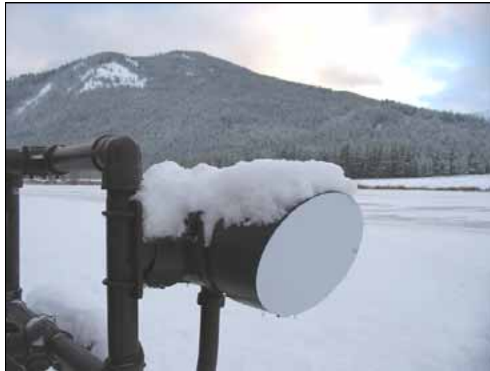
Figure 6.10: Placing a smooth surface at an angle in front of the sensors prevented snow and ice build-up on the sensors at the MT site (Photo: Marcel Huijser, WTI-MSU)
