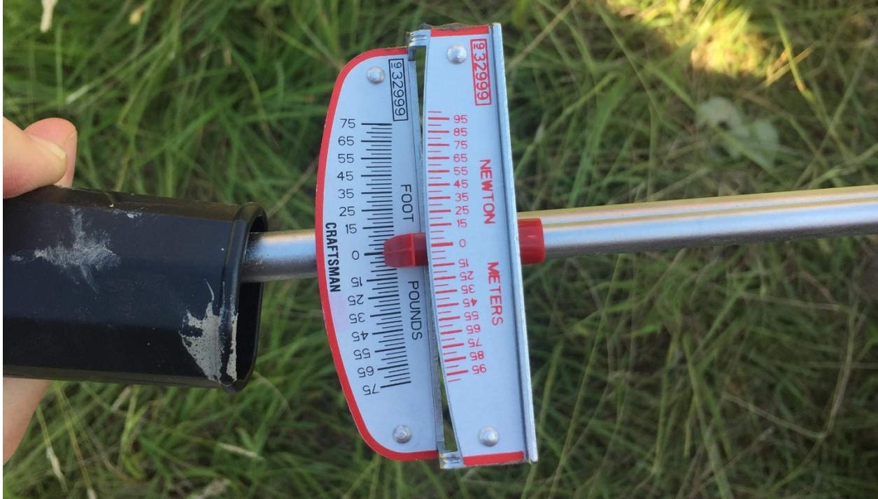
Figure 3.7. Photograph showing the scale used to measure torque mobilized by the vane (photo shows pre-rotation null torque).
