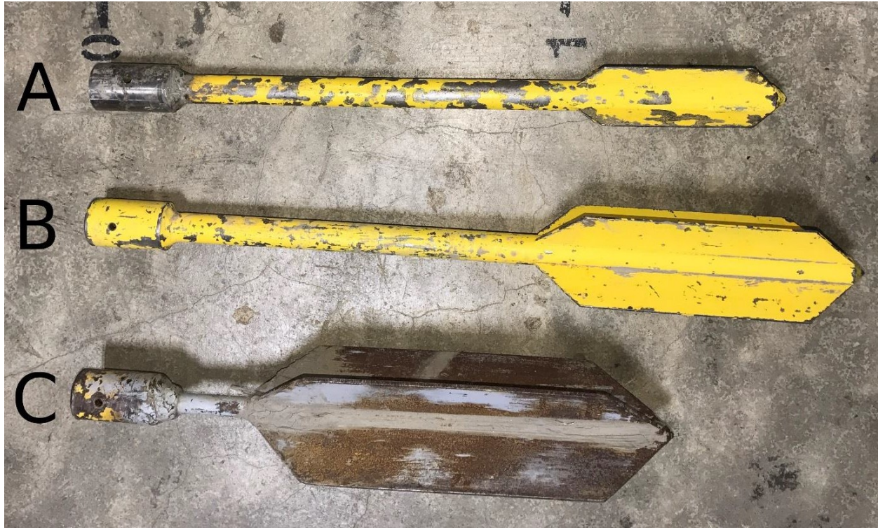
Figure 3.6. Photograph showing Vanes A, B, and C evaluated in the field for determination of the undrained shear strength.
