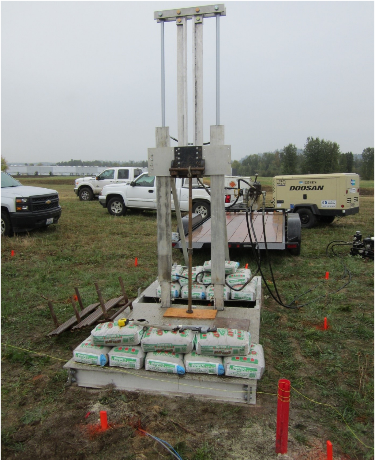
Figure 4.5. Weighted skid rig pre-positioned over borehole V-2 with 8 m (27 ft.) of CPT rod and VST attachment suspended over the base of the borehole just prior to the 30 second blast experiment.
