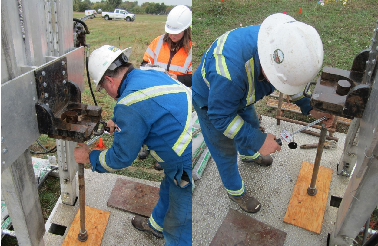
Figure 4.7. Photographs of post-blast VSTs in progress with manually-operated torque wrench. Each VST was observed and time noted in synchronization with the data acquisition system used to monitor the excess pore pressures.
