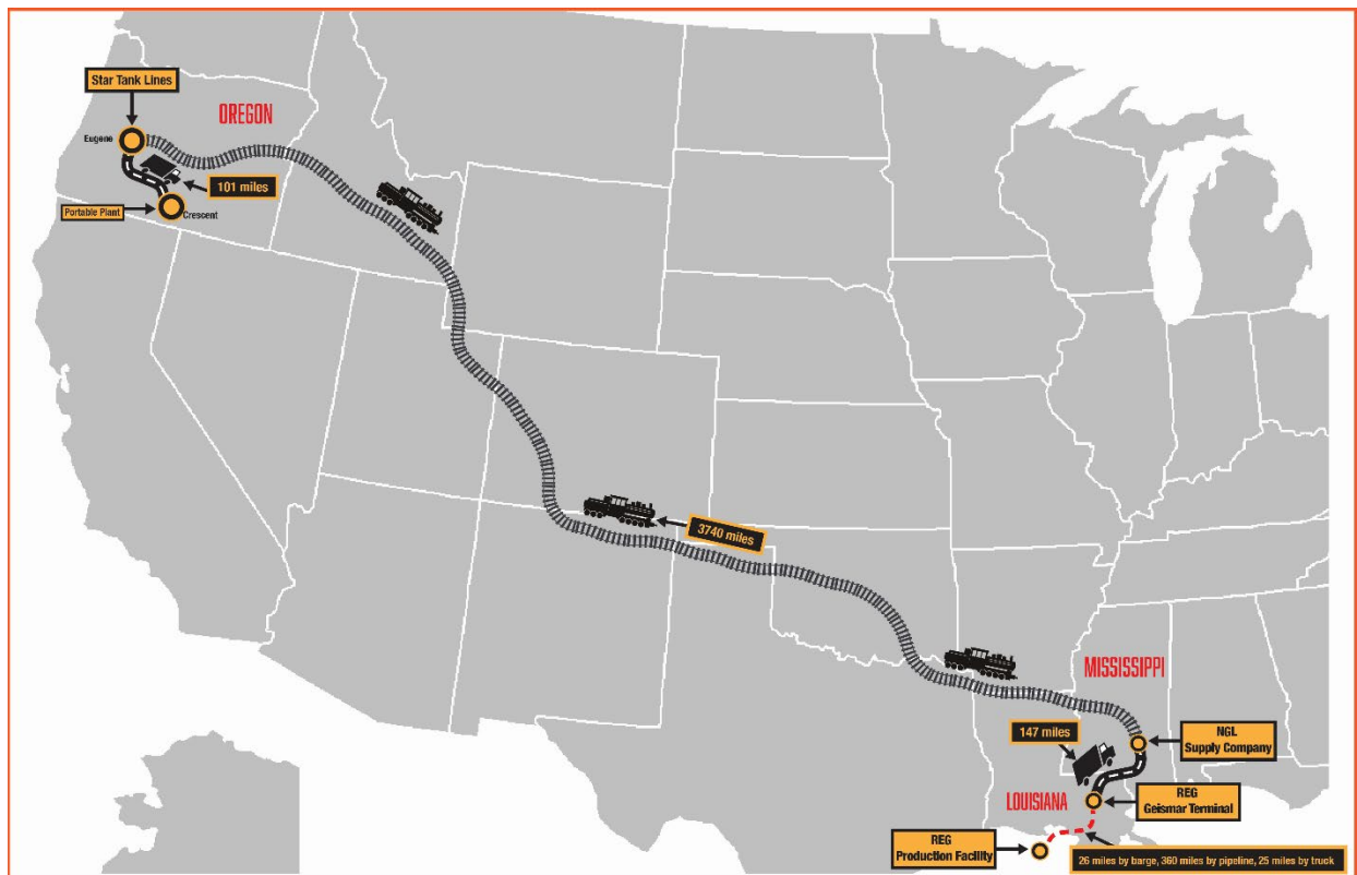
Figure 1. The transportation path for the renewable propane used for the pilot asphalt production in Crescent, Oregon.
