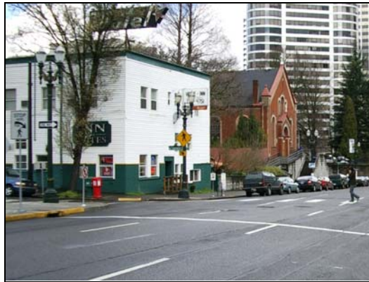
Figure 5.20: Advanced stop bar for cross walk
