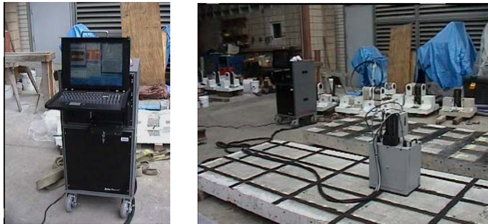
Figure 9.7: a) Thermography data acquisition; b) Initial thermography inspection of specimens
