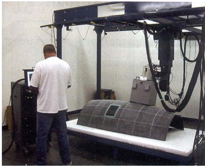
Figure 8.29: Automated thermographic inspection of a composite jet engine cowling [45]
