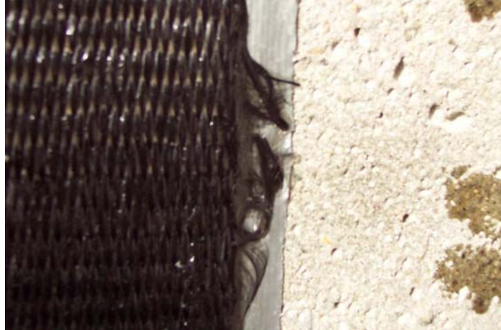
Figure 2.20: Fiber placement over duct tape
