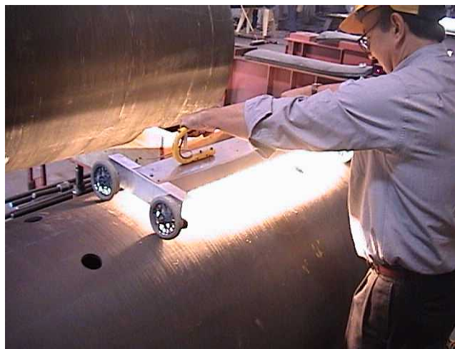
Figure 4.27: Semi-automated heating device
