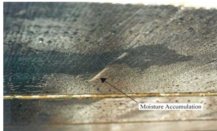
Figure 2.4: Delamination due to entrapped moisture
