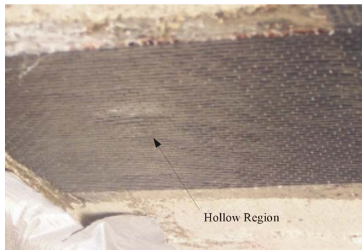
Figure 2.24: Air entrapment over hollow regions
