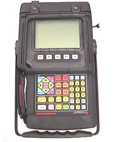
Figure 4.15: Portable UT unit
