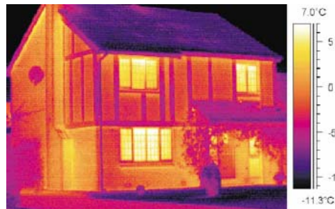
Figure 8.10: Thermography survey of a house for assessment of heat loss [40]
