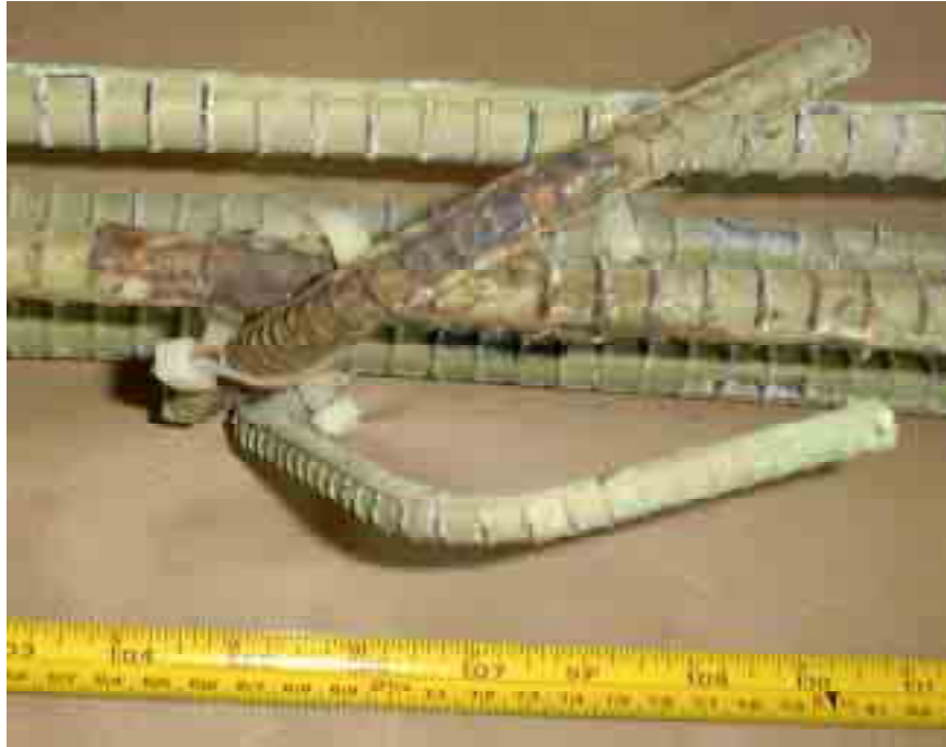
Figure 4.20: Hoop Corrosion in the Tidal Zone
