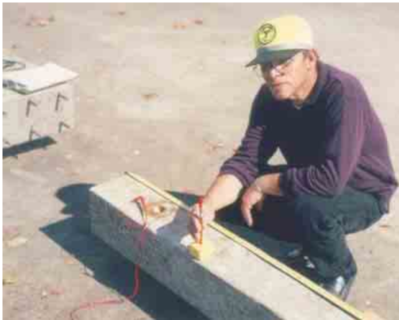
Figure 4.6: Half-Cell Potential Measurements Using Copper-Copper Sulfate Electrode
