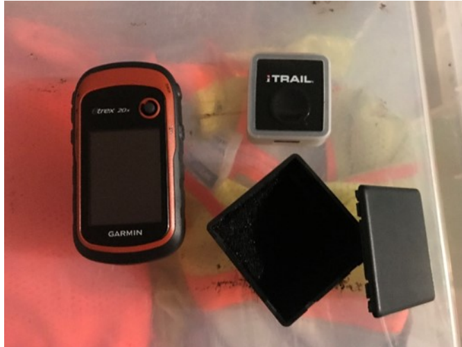
Figure 2.7: Handheld GPS device (left), and GPS tracker and casing for GPS tracker (right)
