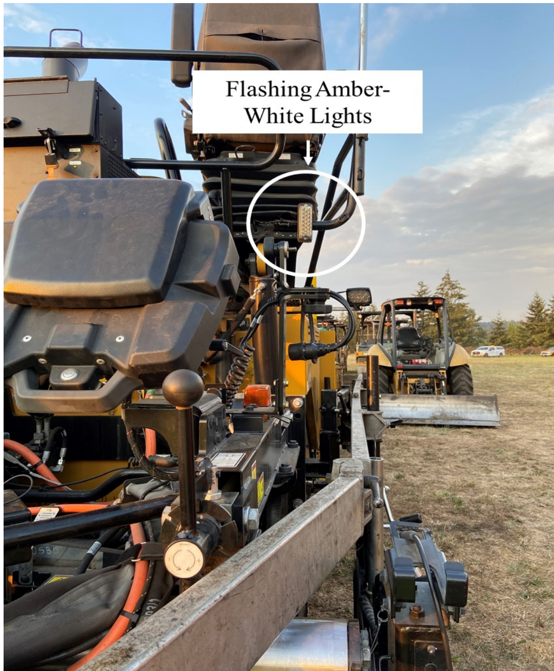
Figure 3.4: Amber-white light installed on paving equipment (case study 2)
