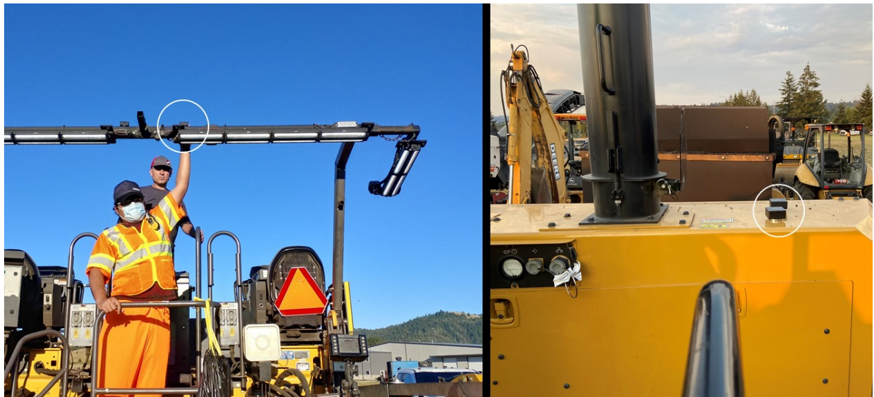
Figure 2.8: GPS sensor location on the paver light bar (left) and on top of paver (right)
