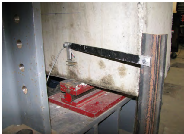
Figure 3.20: Typical vertical displacement sensor to measure support settlement
