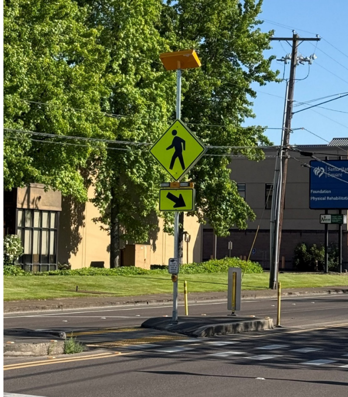
Figure 1-1: Rectangular Rapid Flashing Beacon at NW 9 th St, Corvallis, OR
