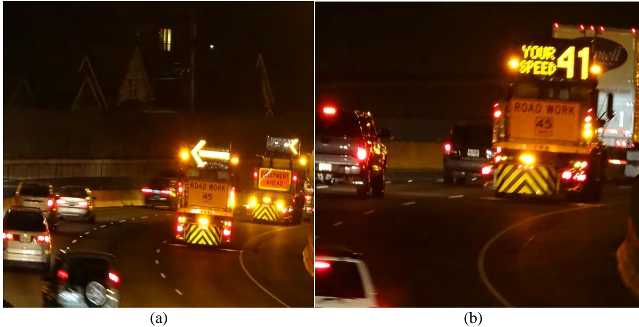
Figure 3.20: Advisory Speed Sign during (a) First Night of Testing and (b) Second Night of Testing (Case Study #3)
