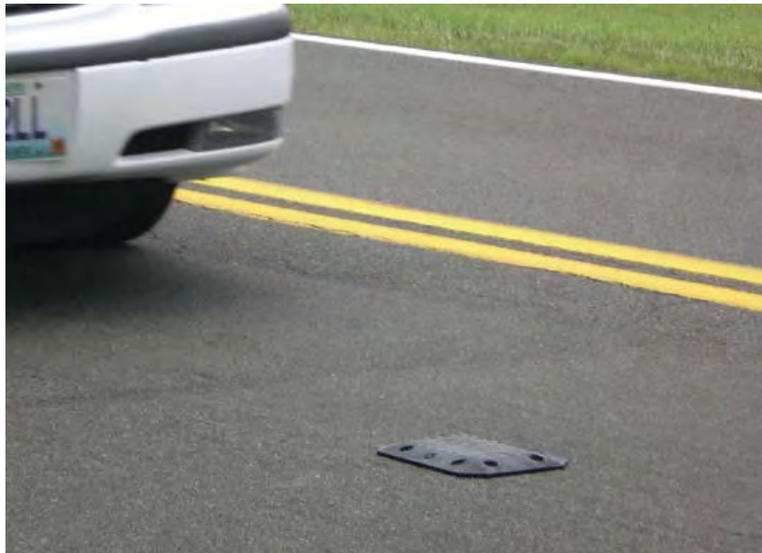
Figure 3.13: Placement of Portable Traffic Analyzer using Nails (Vaisala 2012)
