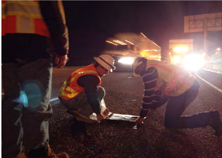
Figure 3.14: Placement of Portable Traffic Analyzer using Adhesive Tape
