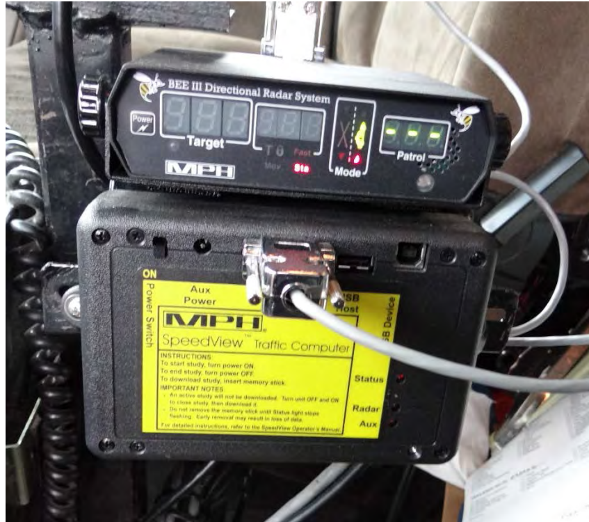
Figure 3.5: SpeedView Traffic Analysis Unit inside Truck Cab
