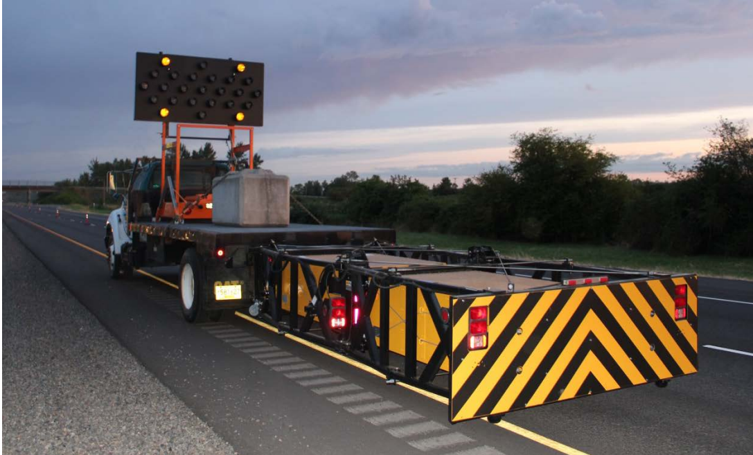
Figure 2.6: Truck Mounted Attenuator and Sequential Arrow Board
