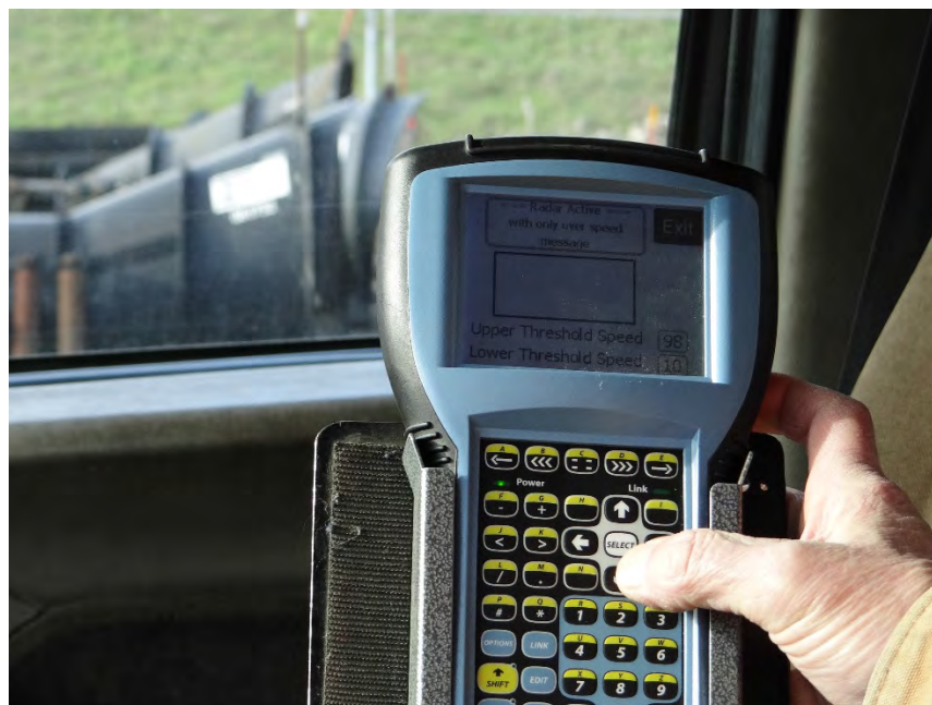
Figure 3.4: Radar System Keyboard inside Truck Cab
