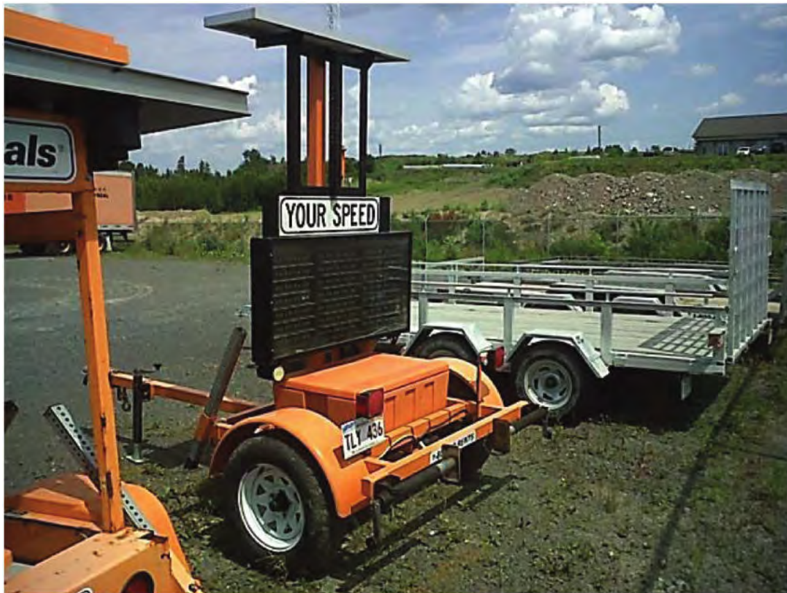
Figure 2.14: Radar Speed Display Board ( Hildebrand and Mason 2014 )
