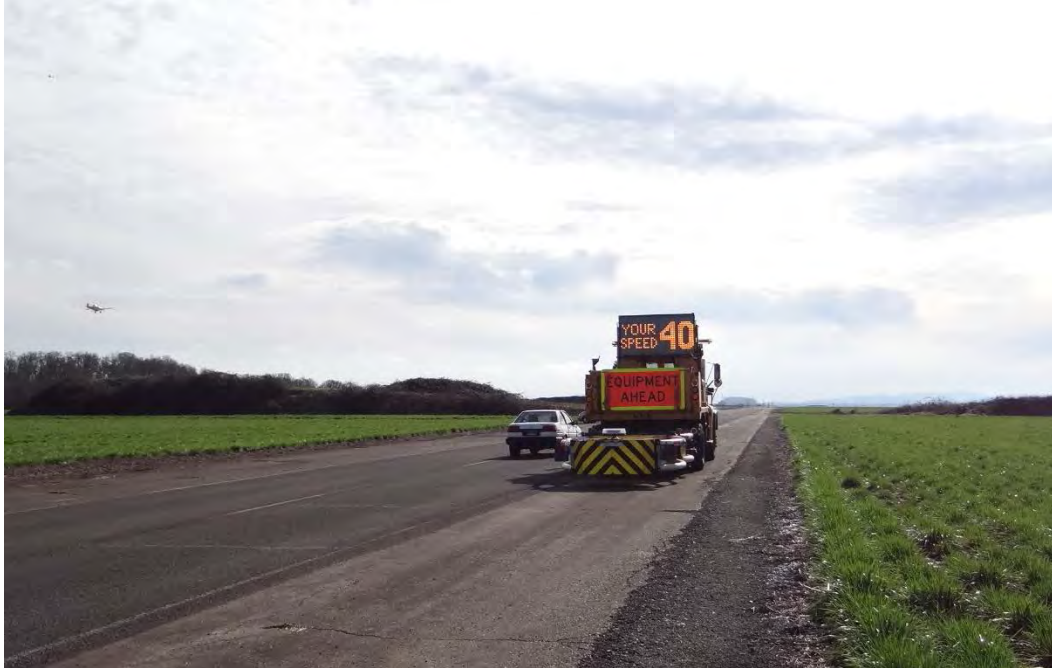
Figure 3.1: Truck-Mounted Radar Speed Display
