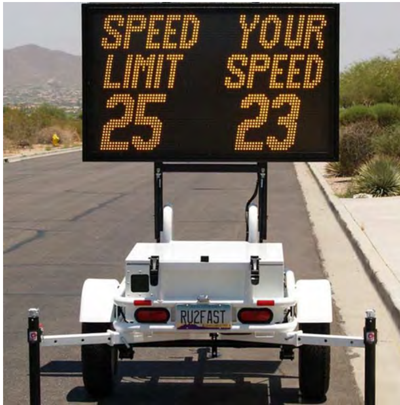
Figure 2.9: Radar Speed Trailer
