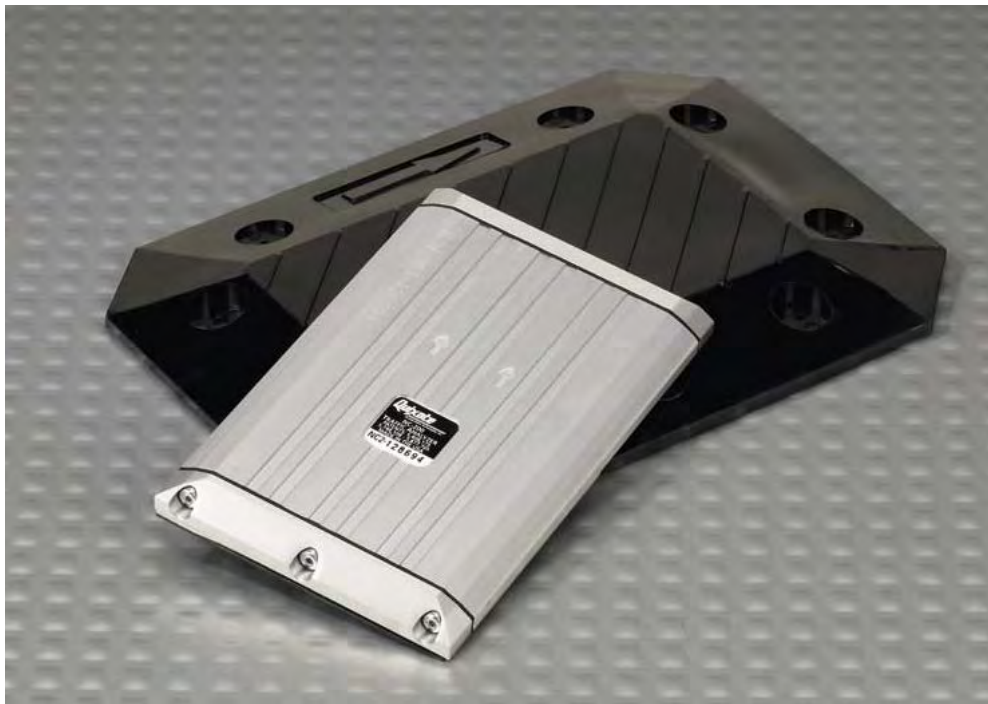
Figure 3.12: Portable Traffic Analyzer NC-200 (Vaisala 2012)
