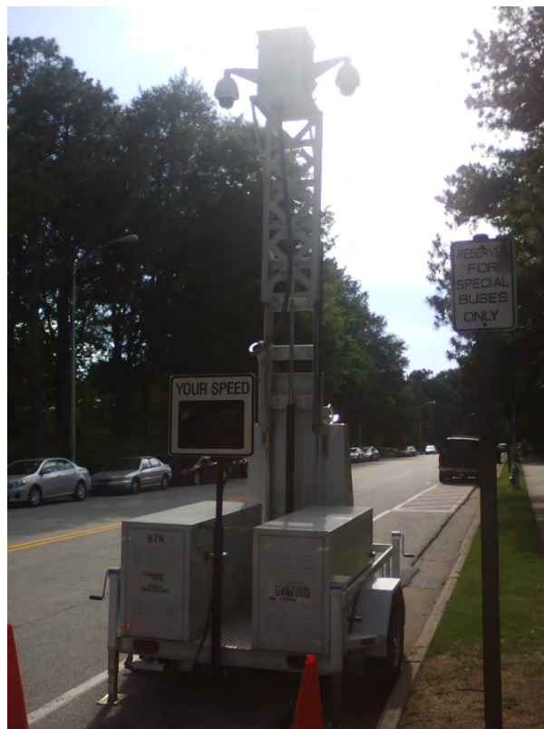
Figure 2.13: Photo Enforcement Equipment
