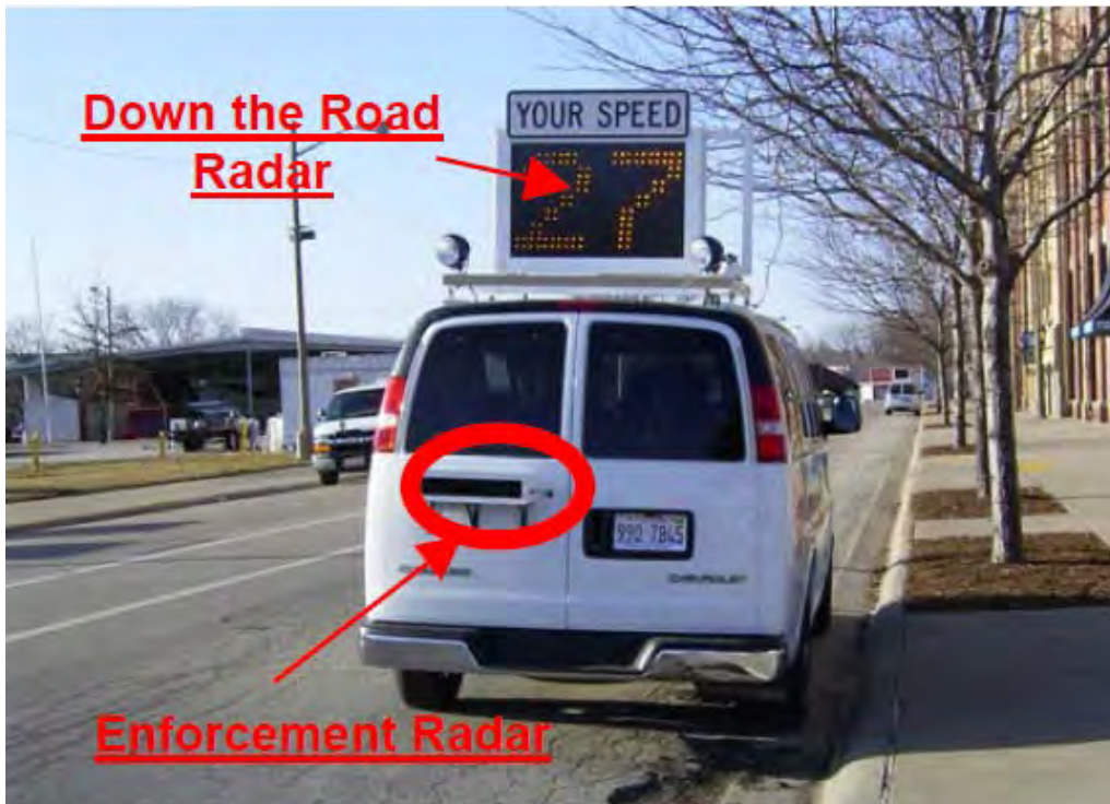
Figure 2.11: Photo Enforcement Vehicle ( Benekohal et al. 2010 )
