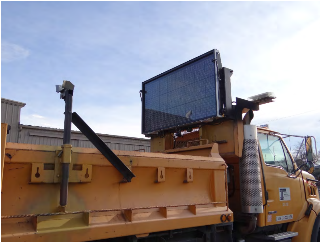
Figure 3.2: 1030F-4W-1 Full Matrix Speed Display
