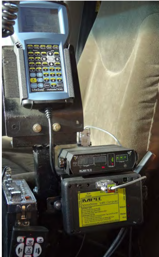
Figure 3.3: Radar Speed Display Units inside Truck Cab
