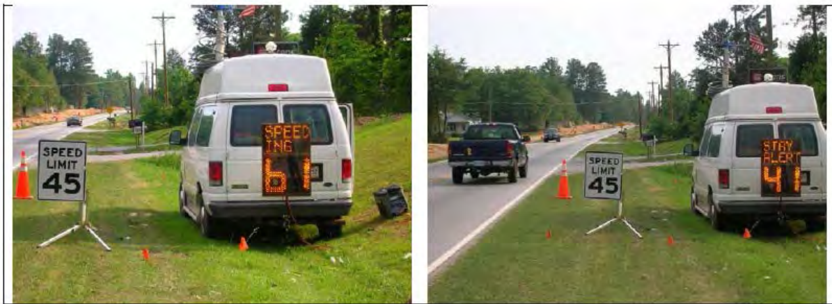
Figure 2.17: Setup Showing Speed Triggered Message and Continuous Message
