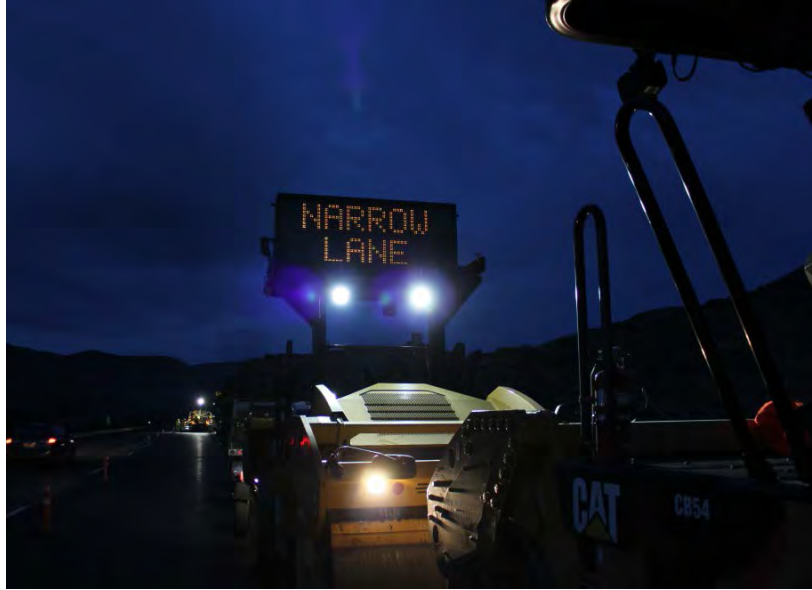
Figure 2.8: PCMS on Roller
