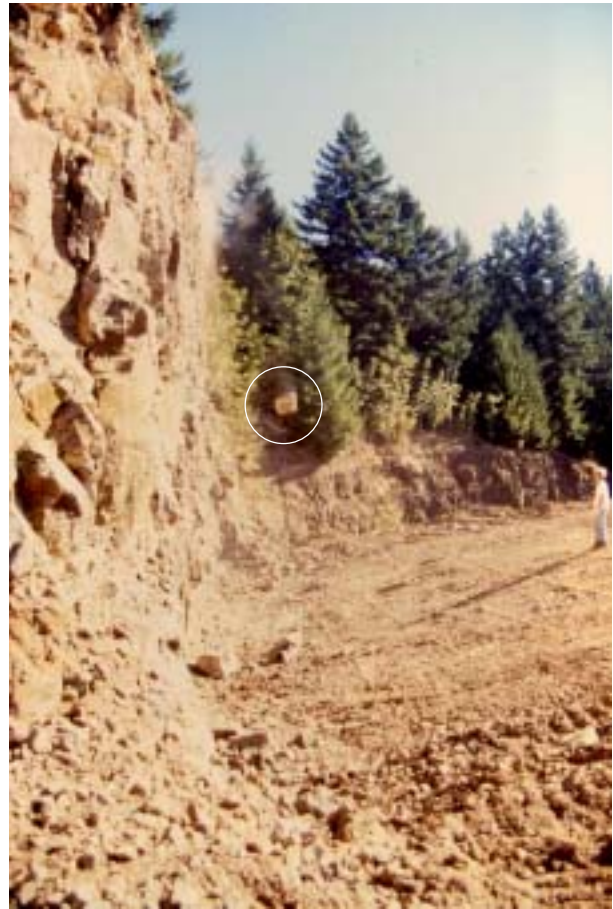
Figure 3.4: Rockfall testing; 12.2-meter high vertical presplit slope. Circle denotes test rock. Grid lines (middle-right) are for measuring impact and roll out distances.
