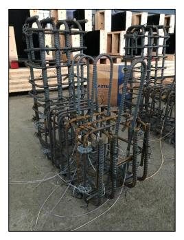
Figure 3.17: Cage for a specimen containing #4 (#13M) reinforcing bars across the interface
