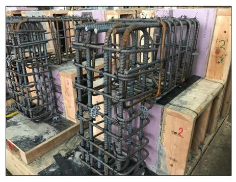
Figure 3.22: Top L-shaped cage is placed on top of specimen
