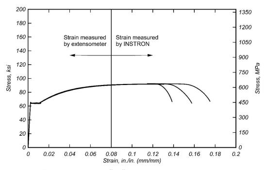
Figure 4.1: Stress-strain plot of #4 (#13M) A706 Grade 60 reinforcing steel bar
