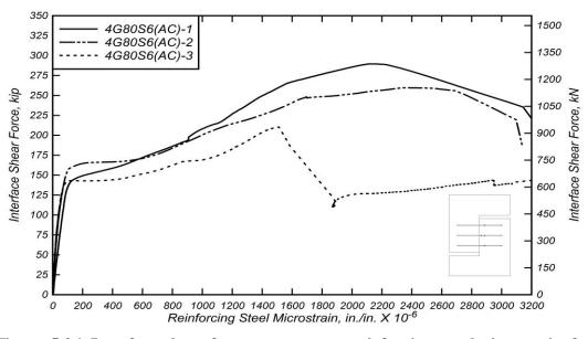
Figure 5.26: Interface shear force versus mean reinforcing steel microstrain for 4G80S6(AC) specimens
