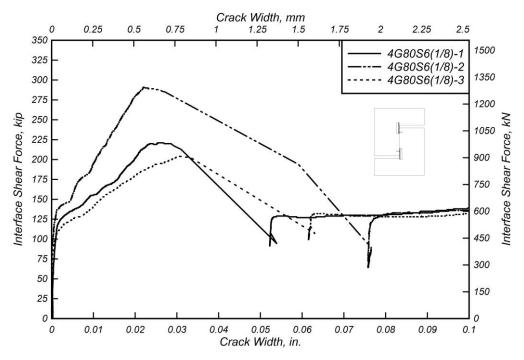
Figure 6.18: Interface shear force versus crack width for 4G80S6(1/8) specimens.
