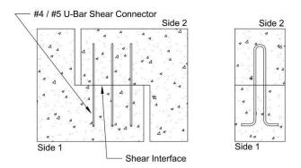
Figure 3.2: Simplified elevation schematic of push-off test specimen containing 3 U-bars to show side 2 (top), side 1 (bottom), reinforcing steel bars, and shear interface
