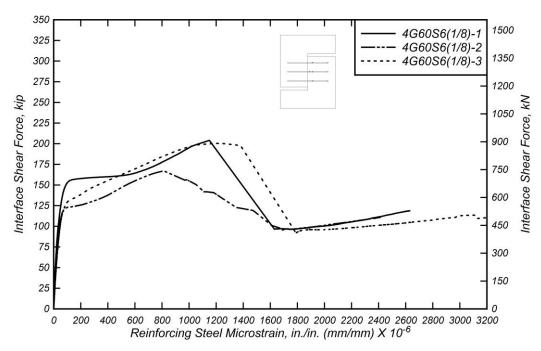
Figure 5.5: Interface shear force versus mean reinforcing steel microstrain for 4G60S6(1/8) specimens
