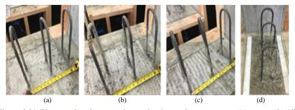
Figure 3.21: Photographs of cast specimens showing surface treatment: (a) as cast, (b) 1/8 in, (c) 1/4 in, and (d) exposed aggregate.
