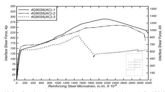
Figure 6.9: Interface shear force versus mean reinforcing steel microstrain for 4G80S6(AC) specimens.
