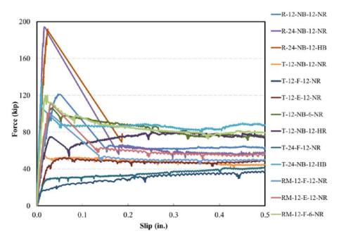
Figure 2.18: Force vs slip (Li et al. 2017) [1 in = 25.4mm]
