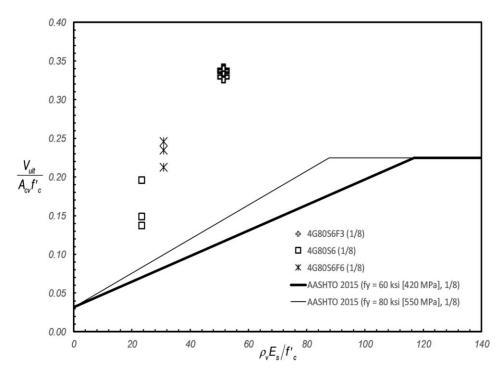
Figure 6.36: Experimental normalized peak shear stress versus normalized reinforcement stiffness across the interface – influence of nominal concrete strength.
