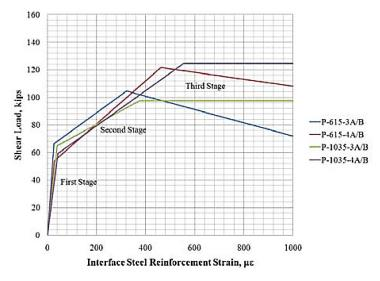
Figure 2.15: Linearization of shear load versus mean interface steel strain showing described stages of the shear friction mechanism (Zeno 2009) [1 kip = 4.448 kN]
