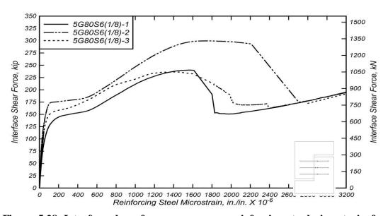
Figure 5.28: Interface shear force versus mean reinforcing steel microstrain for 5G80S6(1/8) specimens
