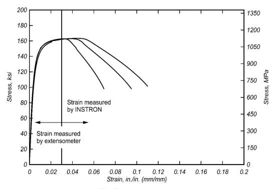
Figure 4.8: Stress-strain plot of #5 (#16M) A1035 CM Grade 120 reinforcing steel bar
