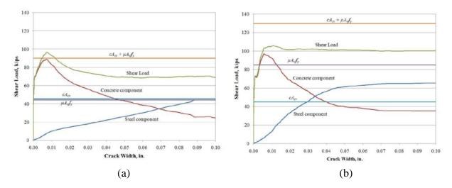
Figure 2.11: Components of shear-friction shear load vs crack width for specimens with reinforcing steel bars consisting of (a) A615 #3 (#10M), and (b) A1035 #3 (#10M) (Zeno (2009))
