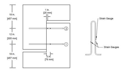
Figure 3.12: Internal instrumentation elevation for specimens built with two U-bars.
