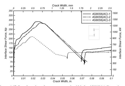
Figure 6.17: Interface shear force versus crack width for 4G80S6(AC) specimens.
