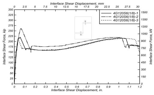
Figure 5.4: Interface shear force versus interface shear displacement for 4G120S6(1/8) specimens
