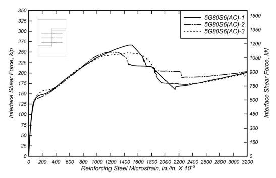
Figure 5.27: Interface shear force versus mean reinforcing steel microstrain for 5G80S6(AC) specimens
