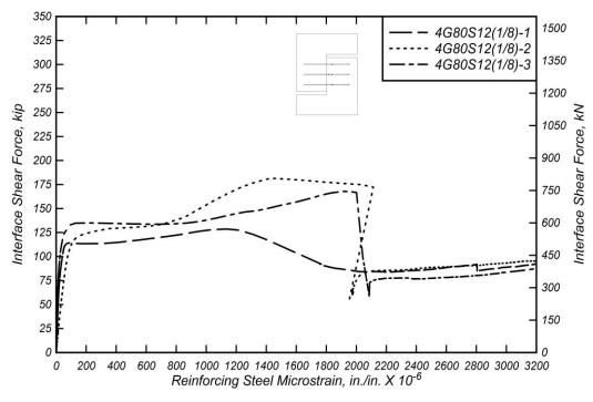
Figure 5.16: Interface shear force versus mean reinforcing steel microstrain for 4G80S12(1/8) specimens
