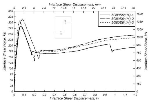
Figure 6.7: Interface shear force versus interface shear displacement for 5G80S6(1/4) specimens.
