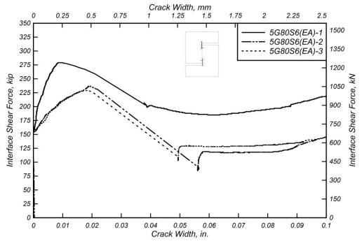
Figure 6.24: Interface shear force versus crack width for 5G80S6(EA) specimens.
