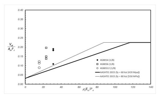
Figure 5.41: Experimental normalized peak shear stress versus normalized reinforcement stiffness across the interface – influence of reinforcing steel bar spacing.
