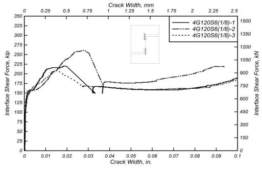
Figure 5.12: Interface shear force versus crack width for 4G120S6(1/8) specimens
