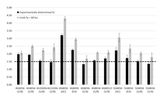
Figure 5.43: Comparison of experimentally measured strength with AASHTO (2015) calculated strength
