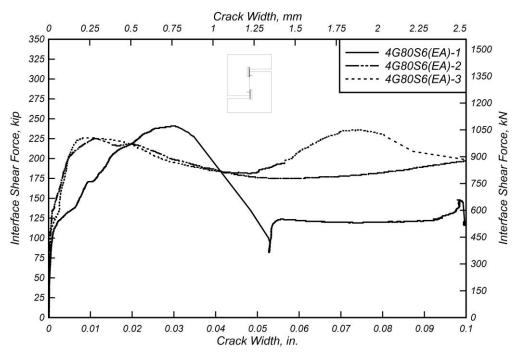
Figure 6.20: Interface shear force versus crack width for 4G80S6(EA) specimens.
