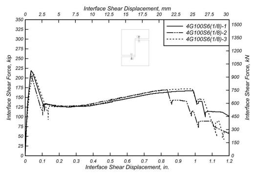
Figure 5.3: Interface shear force versus interface shear displacement for 4G100S6(1/8) specimens.
