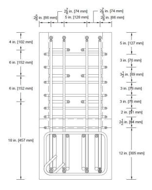
Figure 3.5: Section A-A steel layout for a specimen containing three #4 U-bars spaced at 6 in. (152 mm)
