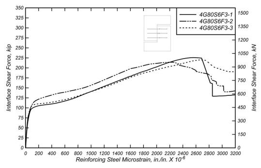
Figure 6.28: Interface shear force versus mean values of reinforcing steel microstrain for 4G80S6F3(1/8) specimens.
