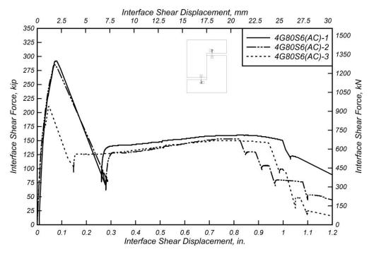
Figure 6.1: Interface shear force versus interface shear displacement for 4G80S6(AC) specimens.
