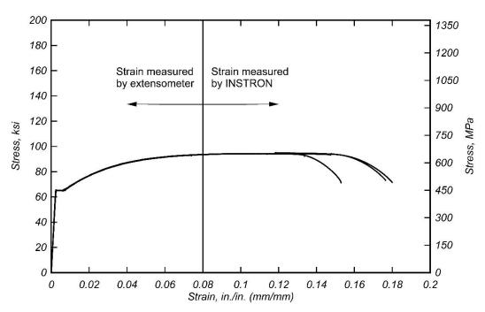
Figure 4.2: Stress-strain plot of #5 (#16M) A706 Grade 60 reinforcing steel bar
