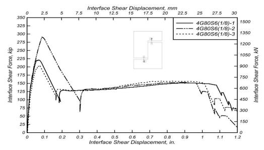
Figure 6.26: Interface shear force versus interface shear displacement the 4G80S6(1/8) specimens.
