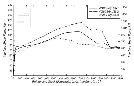
Figure 6.10: Interface shear force versus mean reinforcing steel microstrain for 4G80S6(1/8) specimens.
