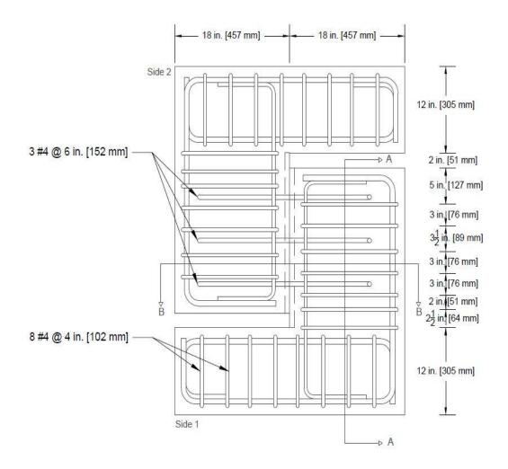
Figure 3.4: Steellayout for a specimen containing three #4 U-bars spaced at 6 in. (152 mm)
