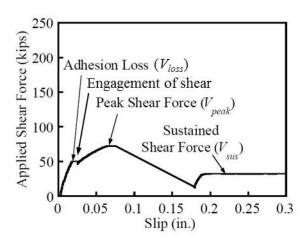
Figure 2.10: Typical failure mode and the plot of the system (Graph recreated from Trejo and Kim 2011)
