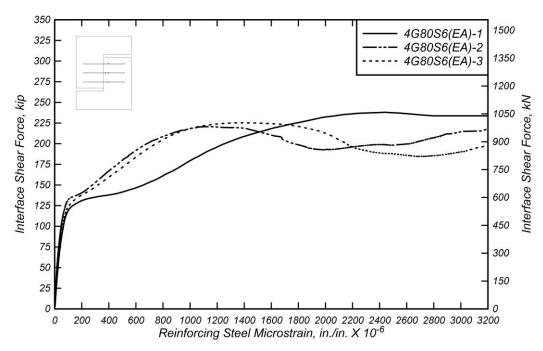
Figure 6.12: Interface shear force versus mean reinforcing steel microstrain for 4G80S6(EA) specimens.
