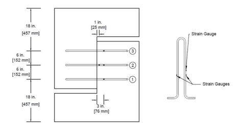
Figure 3.13: Internal instrumentation elevation for specimens built with three U-bars
