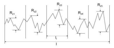
Figure 2.6: Average roughness,  $R_m$ , and mean peak-to-valley height,  $R_z$  (FIB Model Code 2010)
