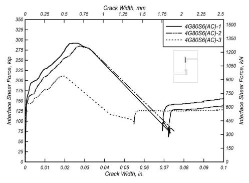
Figure 5.33: Interface shear force versus crack width for 4G80S6(AC) specimens
