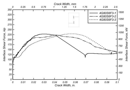
Figure 6.31: Interface shear force versus crack width for 4G80S6F3(1/8) specimens.
