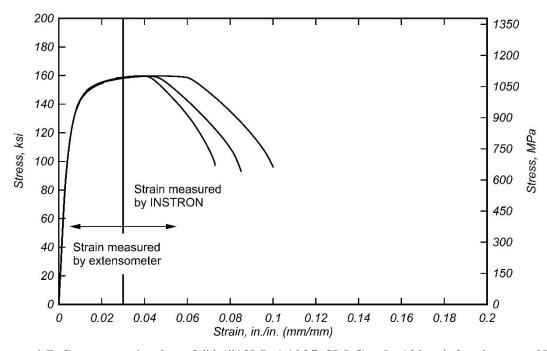
Figure 4.7: Stress-strain plot of #4 (#13M) A1035 CM Grade 120 reinforcing steel bar
