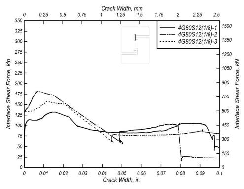
Figure 5.18: Interface shear force versus crack width for 4G80S12(1/8) specimens
