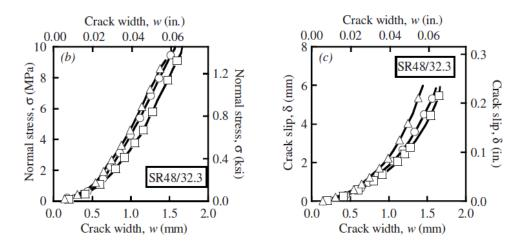
Figure 2.3: Typical plots of measured parameters in interface shear friction tests. Results presented are from Kim et al. (2010), and SR48/32.3 corresponds to a mixture tested that is a self-consolidated [S] concrete mixture, with river gravel [R], 48 MPa strength, and 32.3% coarse aggregate volume.
