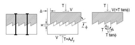
Figure 2.1: Shear friction reinforcement analogy (adapted from Birkeland and Birkeland, 1966)
