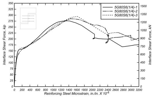
Figure 6.15: Interface shear force versus mean reinforcing steel microstrain for 5G80S6(1/4) specimens.
