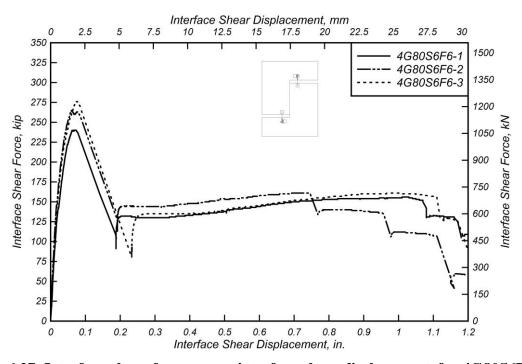
Figure 6.27: Interface shear force versus interface shear displacement for 4G80S6F6(1/8) specimens.
