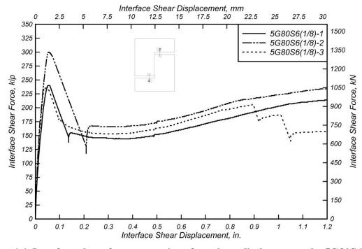
Figure 6.6: Interface shear force versus interface shear displacement the 5G80S6(1/8) specimens.
