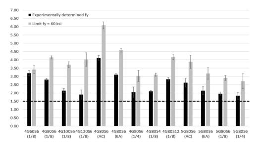
Figure 5.44: Comparison of experimentally measured strength with ACI 318-14 calculated strength
