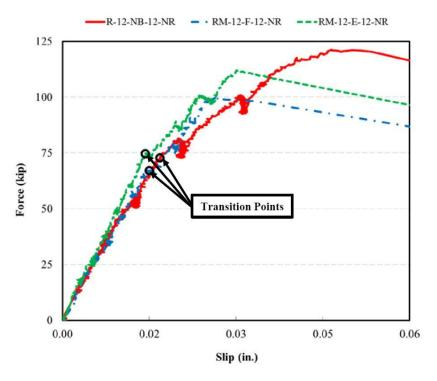
Figure 2.19: Force vs slip zoomed region up to 0.06 in. (1.52mm) slip (Li et al. 2017) [1 in = 25.4mm]
