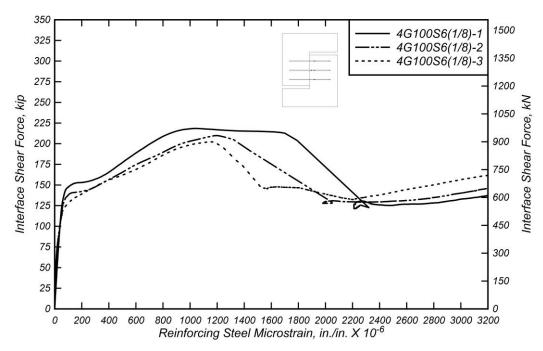
Figure 5.7: Interface shear force versus mean reinforcing steel microstrain for 4G100S6(1/8) specimens
