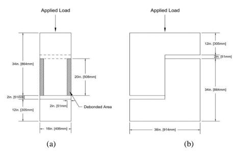
Figure 3.3: (a) Front view elevation, (b) side view elevation
