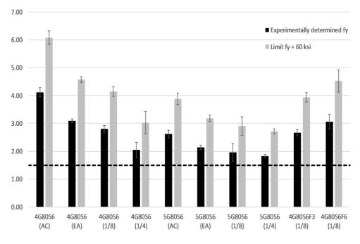
Figure 6.38: Comparison of experimentally measured strength with ACI 318-14 calculated strength.
