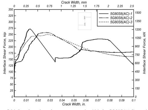
Figure 5.34: Interface shear force versus crack width for 5G80S6(AC) specimens
