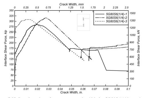
Figure 5.37: Interface shear force versus crack width for 5G80S6(1/4) specimens
