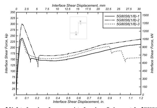
Figure 5.21: Interface shear force versus interface shear displacement for 5G80S6(1/8) specimens.
