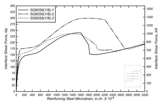
Figure 6.14: Interface shear force versus mean reinforcing steel microstrain for 5G80S6(1/8) specimens.
