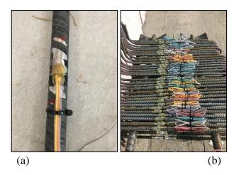
Figure 3.15: Strain gauges applied to U-bar reinforcing (a) view of strain gauge with initial protective coating and (b) view of U-bars after strain gauges are installed
