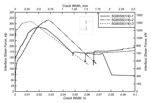
Figure 6.23: Interface shear force versus crack width for 5G80S6(1/4) specimens.
