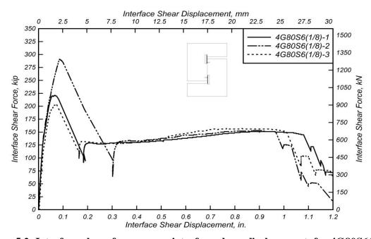
Figure 5.2: Interface shear force versus interface shear displacement for 4G80S6(1/8) specimens
