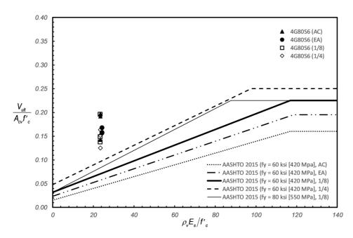
Figure 6.34: Experimental normalized peak shear stress versus normalized reinforcement stiffness across the interface – influence of interface preparation #4 (#13M) reinforcing steel bars.
