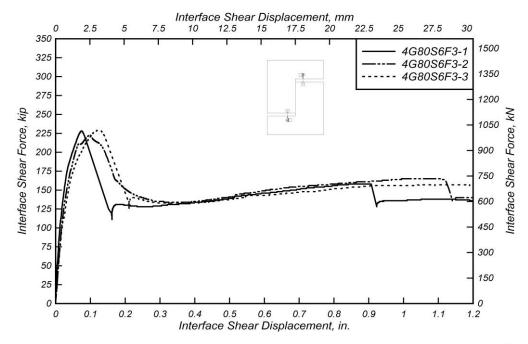
Figure 6.25: Interface shear force versus interface shear displacement for 4G80S6F3(1/8) specimens.
