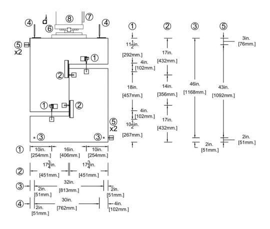
Figure 3.11: North-south external instrumentation elevation view
