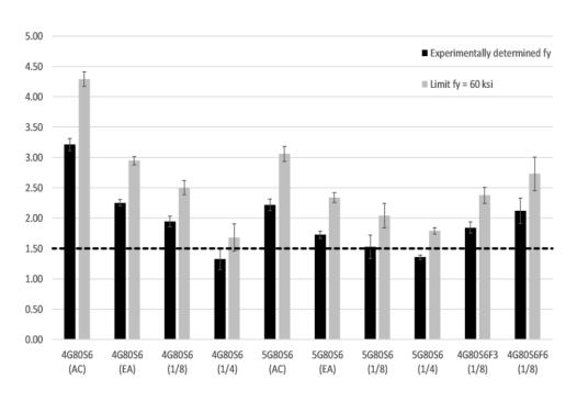
Figure 6.37: Comparison of experimentally measured strength with AASHTO (2015) calculated strength.
