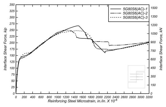
Figure 6.13: Interface shear force versus mean reinforcing steel microstrain for 5G80S6(AC) specimens.
