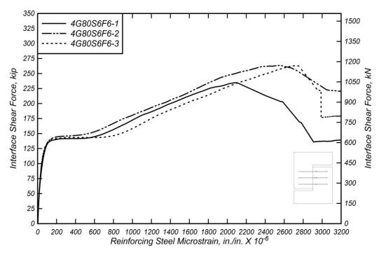
Figure 6.30: Interface shear force versus mean values of reinforcing steel microstrain for 4G80S6F6(1/8) specimens.
