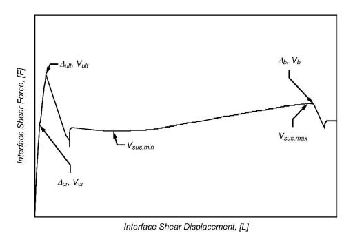
Figure 3.25: Typical force-displacement response of push-off tests and definition of notable parameters.
