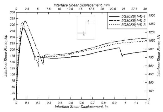
Figure 5.23: Interface shear force versus interface shear displacement for 5G80S6(1/4) specimens
