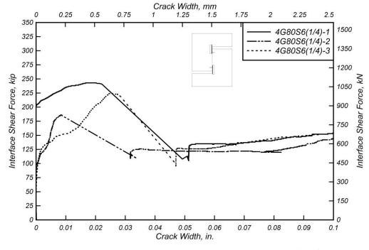
Figure 6.19: Interface shear force versus crack width for 4G80S6(1/4) specimens.
