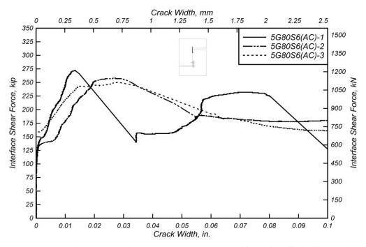
Figure 6.21: Interface shear force versus crack width for 5G80S6(AC) specimens.
