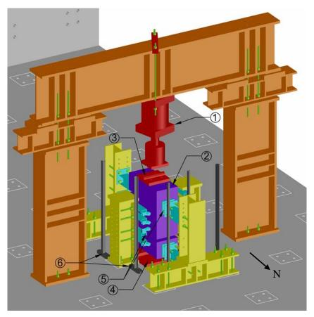
Figure 3.7 General test setup facing southwest. Legend – 1: Actuator; 2: test specimen; 3:roller plate; 4: base plate; 5: roller support for safety (gap provided between rollers and specimen); 6: LVDT sensor supports
