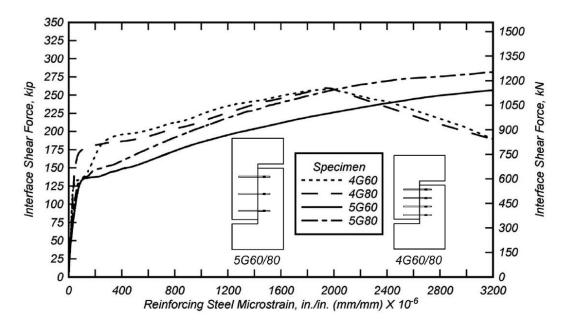
Figure 2.16: Interface shear force versus reinforcing steel strain (Barbosa et al. 2017)
