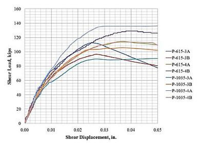
Figure 2.12: Shear load versus shear displacement showing the described stages of the shear friction mechanism (Zeno 2009) [1 in. = 25.4 mm]
