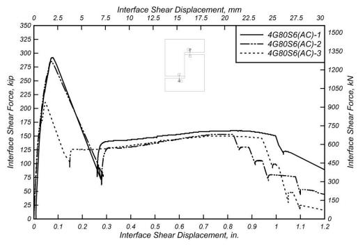
Figure 5.19: Interface shear force versus interface shear displacement for 4G80S6(AC) specimens
