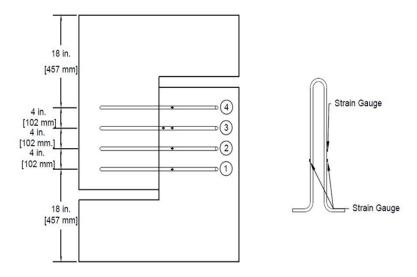
Figure 3.14: Internal instrumentation elevation for specimens built with four U-bars.
