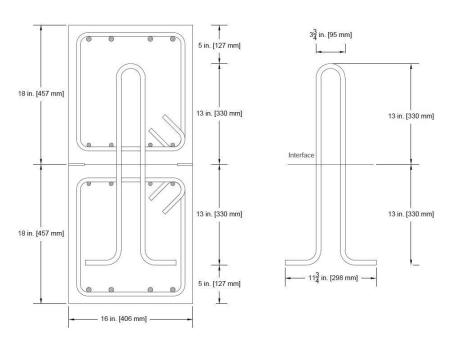
Figure 3.6: Section B-B steellayout for a specimen containing three #4 U-bars spaced at 6 in. (152 mm).
