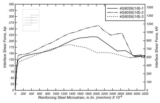
Figure 5.6: Interface shear force versus mean reinforcing steel microstrain for 4G80S6(1/8) specimens
