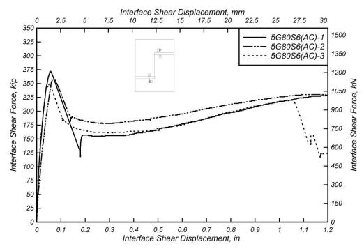
Figure 6.5: Interface shear force versus interface shear displacement for 5G80S6(AC) specimens.
