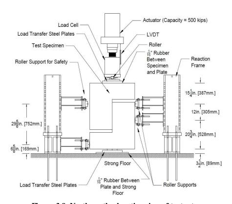
Figure 3.9: North-south elevation view of test setup
