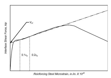
Figure 3.26: Illustration of the points used to determine the point of loss of cohesion.
