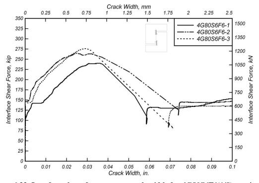
Figure 6.33: Interface shear force versus crack width for 4G80S6F6(1/8) specimens.
