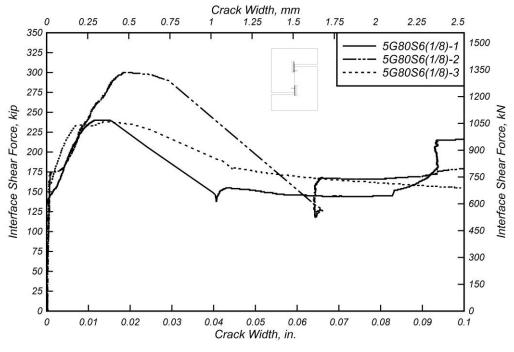
Figure 6.22: Interface shear force versus crack width for 5G80S6(1/8) specimens.
