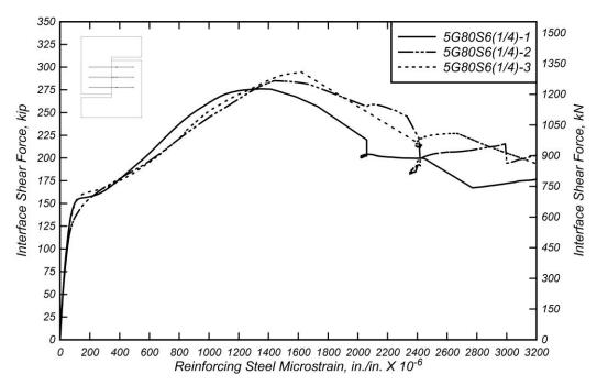
Figure 5.30: Interface shear force versus mean reinforcing steel microstrain for 5G80S6(1/4) specimens.
