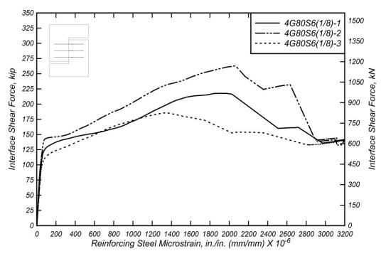
Figure 6.29: Interface shear force versus mean values of reinforcing steel microstrain for 4G80S6(1/8) specimens.
