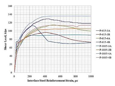
Figure 2.14: Shear load versus mean interface steel strain showing described stages of the shear friction mechanism (Zeno 2009) [1 kip = 4.448 kN]
