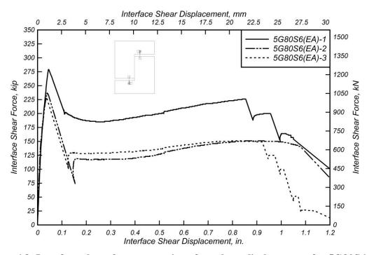
Figure 6.8: Interface shear force versus interface shear displacement for 5G80S6(EA) specimens.
