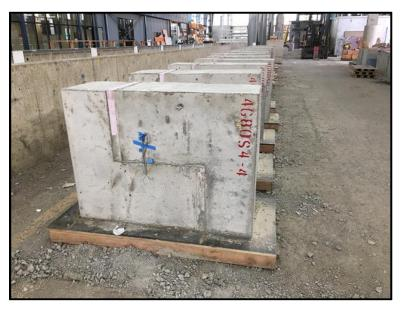
Figure 3.24: Constructed specimens after formwork removal
