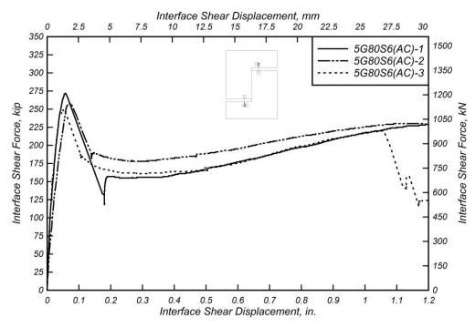
Figure 5.20: Interface shear force versus interface shear displacement for 5G80S6(AC) specimens
