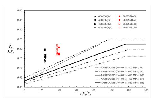
Figure 5.42: Experimental normalized peak shear stress versus normalized reinforcement stiffness across the interface – influence of reinforcing steel bar size.
