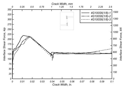
Figure 5.11: Interface shear force versus crack width for 4G100S6(1/8) specimens
