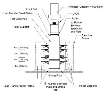
Figure 3.10: East-west elevation view of test setup [1 in. = 25.4mm; 1 kip = 4.48 kN]
