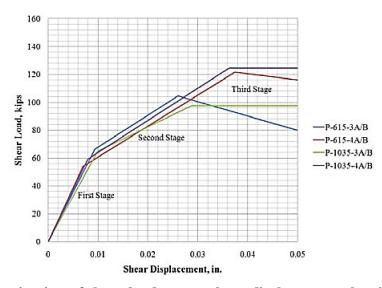
Figure 2.13: Linearization of shear load versus shear displacement showing the described stages of the shear friction mechanism (Zeno 2009) [1 in. = 25.4 mm]
