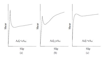
Figure 2.8: Typical Load versus Slip Plots (Wallenfelsz, 2006)
