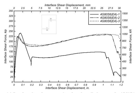
Figure 6.4: Interface shear force versus interface shear displacement for  $4G\,80S6(EA)$  specimens.
