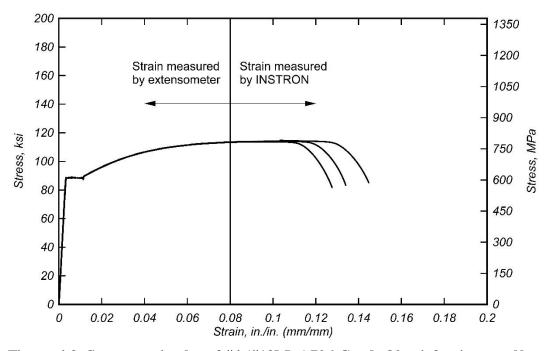
Figure 4.3: Stress-strain plot of #4 (#13M) A706 Grade 80 reinforcing steel bar
