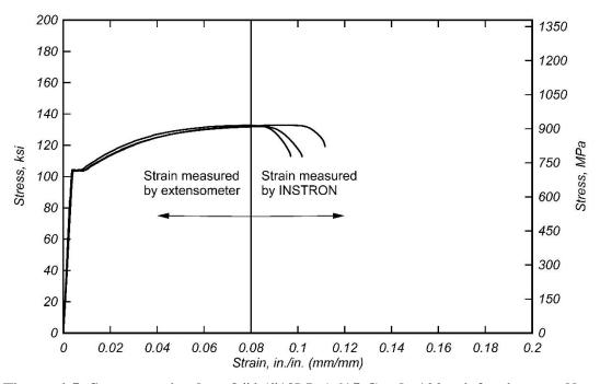
Figure 4.5: Stress-strain plot of #4 (#13M) A615 Grade 100 reinforcing steel bar
