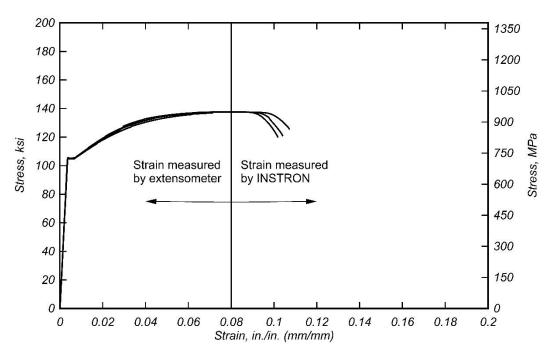
Figure 4.6: Stress-strain plot of #5 (#16M) A615 Grade 100 reinforcing steel bar
