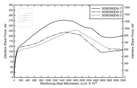
Figure 5.32: Interface shear force versus mean reinforcing steel microstrain for 5G80S6(EA) specimens.
