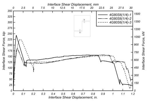
Figure 6.3: Interface shear force versus interface shear displacement for 4G80S6(1/4) specimens.
