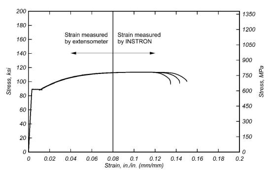
Figure 4.4: Stress-strain plot of #5 (#16M) A706 Grade 80 reinforcing steel bar
