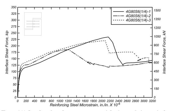
Figure 6.11: Interface shear force versus mean reinforcing steel microstrain for 4G80S6(1/4) specimens.
