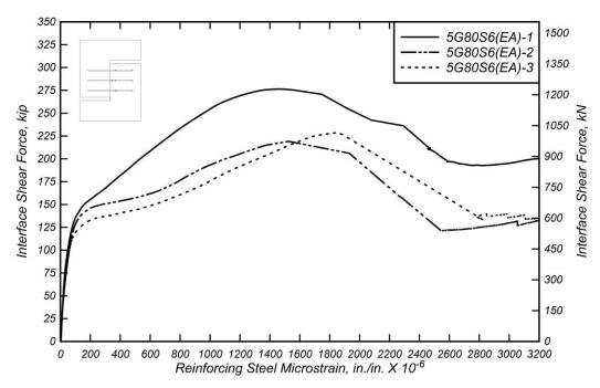
Figure 6.16: Interface shear force versus mean reinforcing steel microstrain for 5G80S6(EA) specimens.
