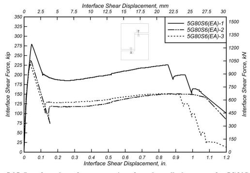
Figure 5.25: Interface shear force versus interface shear displacement for 5G80S6(EA) specimens
