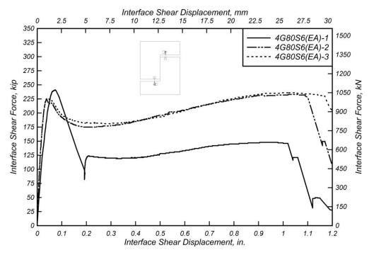
Figure 5.24: Interface shear force versus interface shear displacement for 4G80S6(EA) specimens
