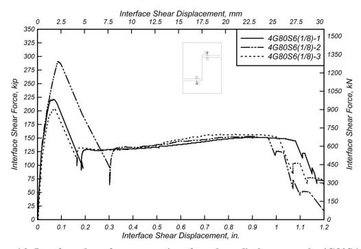
Figure 6.2: Interface shear force versus interface shear displacement the 4G80S6(1/8) specimens.
