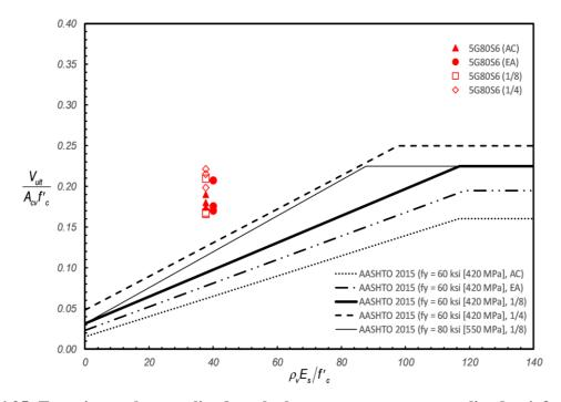
Figure 6.35: Experimental normalized peak shear stress versus normalized reinforcement stiffness across the interface – influence of interface preparation #5 (#16M) reinforcing steel bars.
