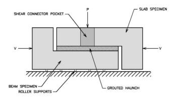
Figure 2.7: Horizontal push-off test (Wallenfelsz, 2006)
