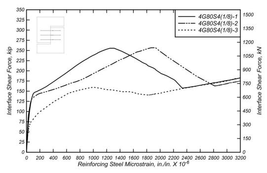
Figure 5.15: Interface shear force versus mean reinforcing steel microstrain for 4G80S4(1/8) specimens
