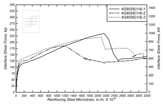
Figure 5.29: Interface shear force versus mean reinforcing steel microstrain for 4G80S6(1/4) specimens.
