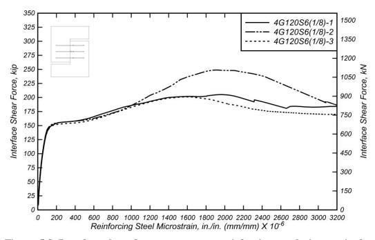
Figure 5.8: Interface shear force versus mean reinforcing steel microstrain for 4G120S6(1/8) specimens
