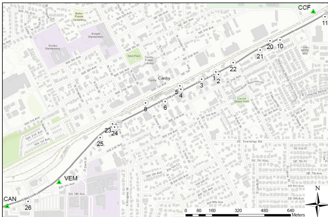
Figure 2.3: Map of control stations utilized in Phase II of this study. This control network is located in Canby, Oregon along Highway 99E and consists of 19 ODOT control marks signified by white circles with black stars and green triangles.
