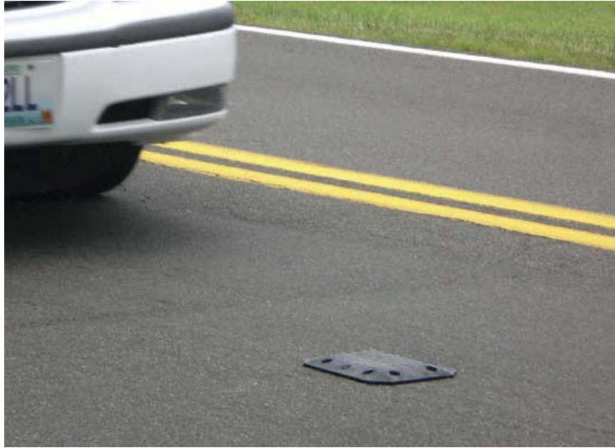
Figure 3.5: Placement of Portable Traffic Analyzer by Nails ( Vaisala 2012 )
